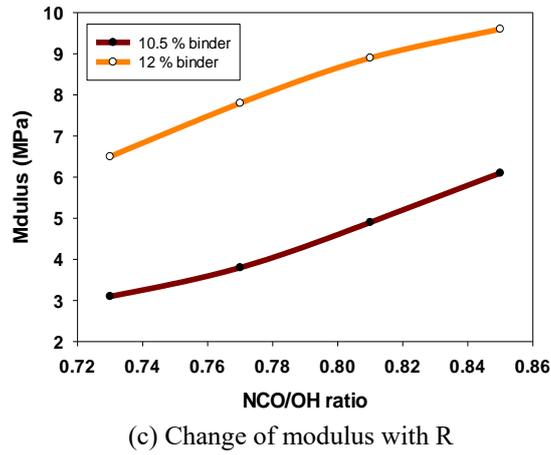
Fig. 2 UTS, elongation and modulus comparison of 10.5% and 12% binder with variation of R
