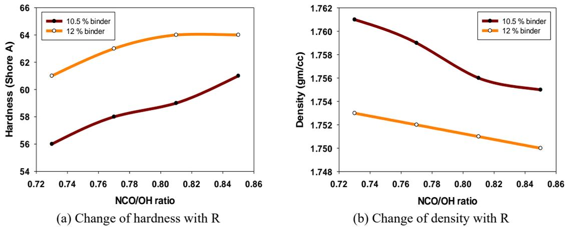
Fig. 3 Hardness and density comparison of 10.5% and 12% binder with variation of R
