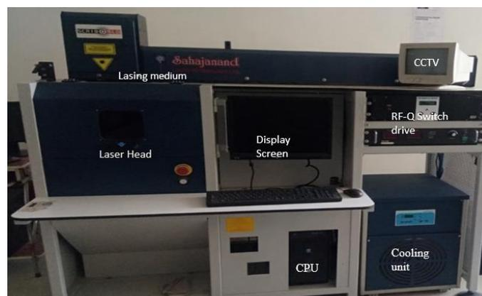
Fig. 1 Nd:YAG laser micro-drilling machine setup
