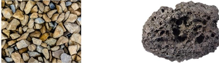
Fig. 2 Limestone aggregate (left) and scoria aggregate (right)
