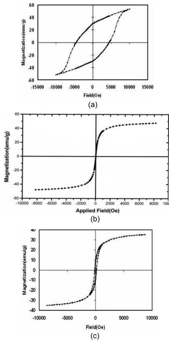
Fig. 5 Magnetic properties of samples (a) nanoflake  $\text{SrFe}_{12}\text{O}_{19}$ , (b)  $\text{Fe}_3\text{O}_4$  nanoparticle, (c) core-shell  $\text{SrFe}_{12}\text{O}_{19}/\text{Fe}_3\text{O}_4$  and (d) nanocomposite  $\text{SrFe}_{12}\text{O}_{19}/\text{Fe}_3\text{O}_4/\text{PEG}/\text{PPy}$
