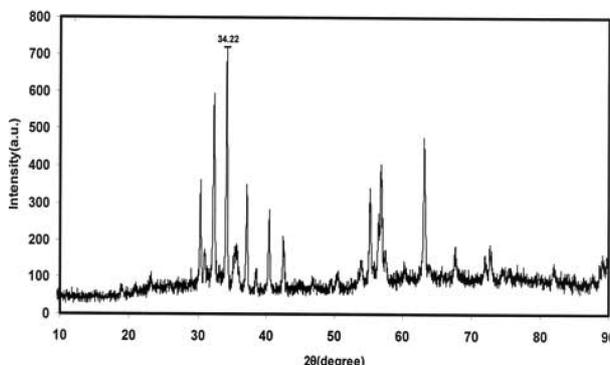
Fig. 1 X-ray diffraction pattern of nanoflake  $\text{SrFe}_{12}\text{O}_{19}$  calcined at  $850^\circ\text{C}$  for 2 h
