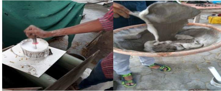
Fig. 3 Preparation of foam and mixing of foam with a wet mix for tile specimen
