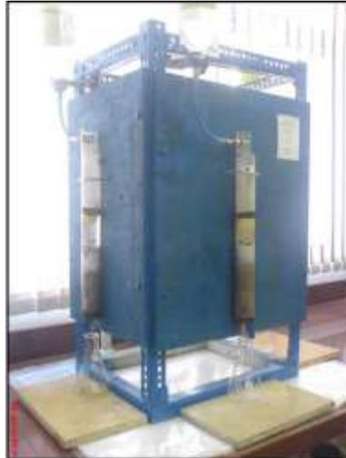
Fig. 1 Sand column apparatus of soil washing process (Salehian 2007)
