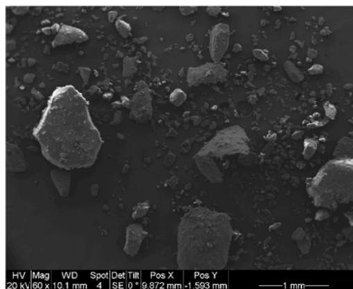
Fig. 2 Scanning Electron microscope (SEM) image of EGMs
