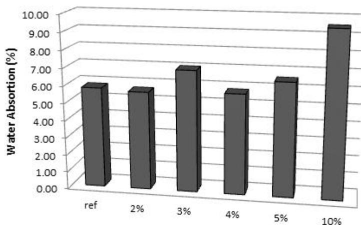
Fig. 2 Water absorption of concrete paving blocks manufactured with blasting dust
