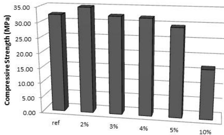
Fig. 1 Characteristic compressive strength of concrete paving blocks with blasting dust
