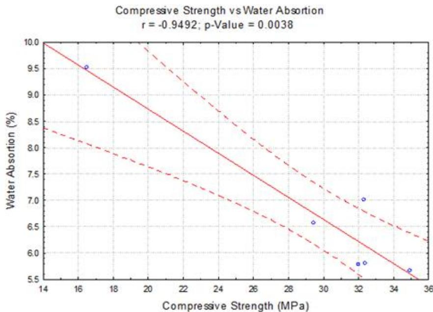
Fig. 3 Scatter plot for water absorption vs. compressive strength
