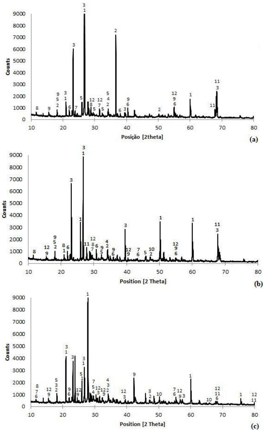
Fig. 4 Diffractograms of concrete block samples manufactured with blasting dust: (a) reference block; (b), (c), (d), (e), (f) blocks manufactured with 2%, 3%, 4% and 5% of electroplating waste, respectively
