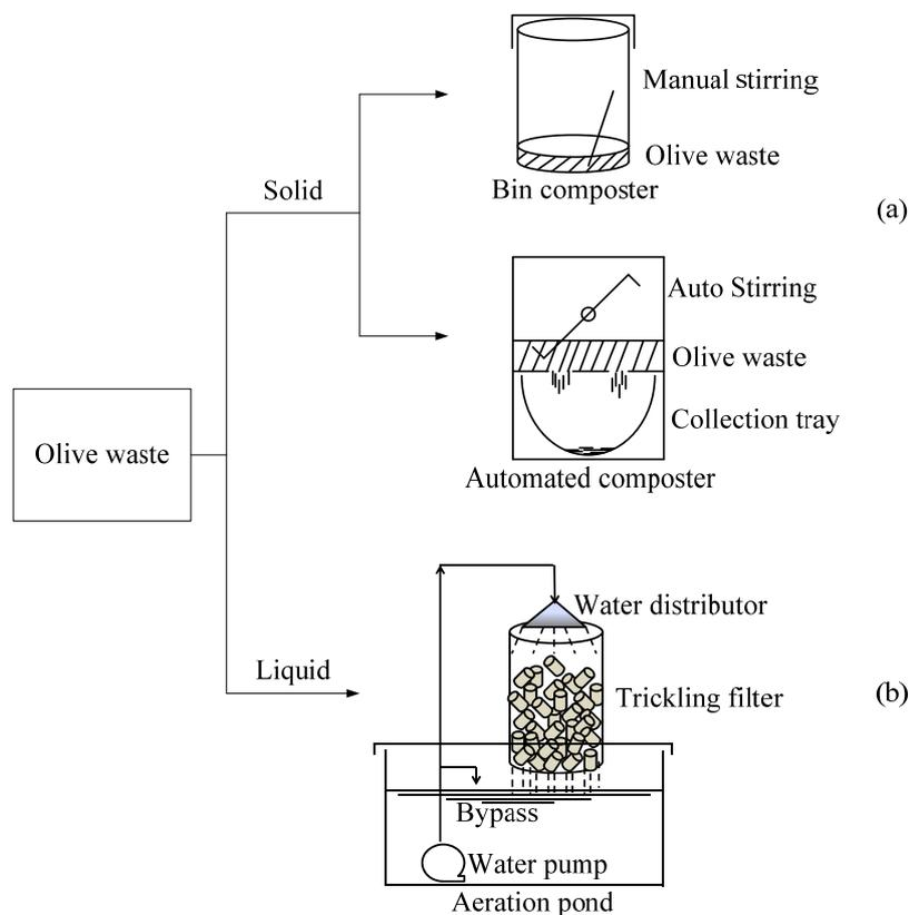
Fig. 1 (a) Composting for OMW solids; (b) Pond/trickling filter for OMW liquid
