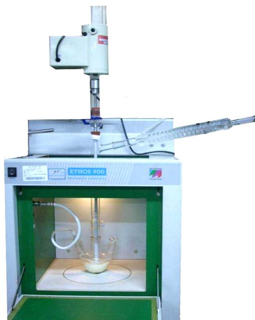
Fig. 1 Modified microwave heating system used for transesterification reactions
