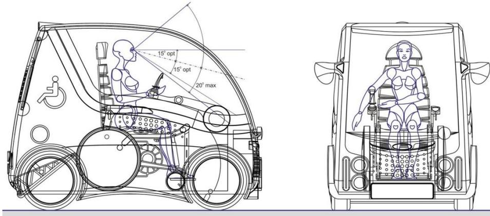
Fig. 7 Ergonomic scheme of the individual vehicle
