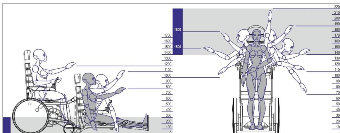
Fig. 6 Ergonomic scheme of the wheelchair
