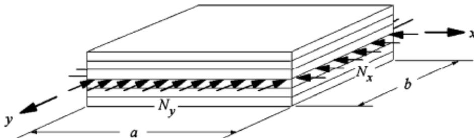
Fig. 1 A symmetric laminate under compressive biaxial loads
