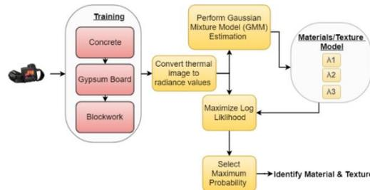
Fig. 4 Workflow for Material and Texture Identification using GMM model
