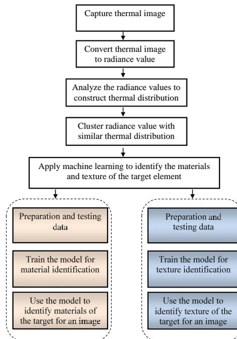
Fig. 2 Materials and texture identification workflow
