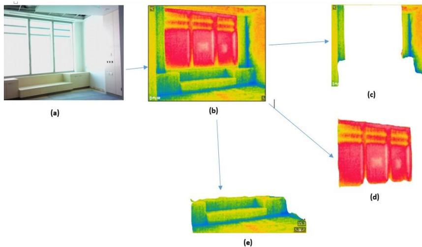
Fig. 8 Texture extraction and feature labeling of an interior gypsum board wall and window in a thermal image
