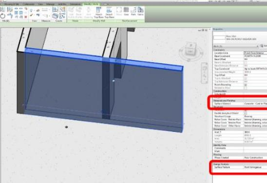
(d) The updated BIM showing concrete surface material and inhomogeneous texture of the interior walls
