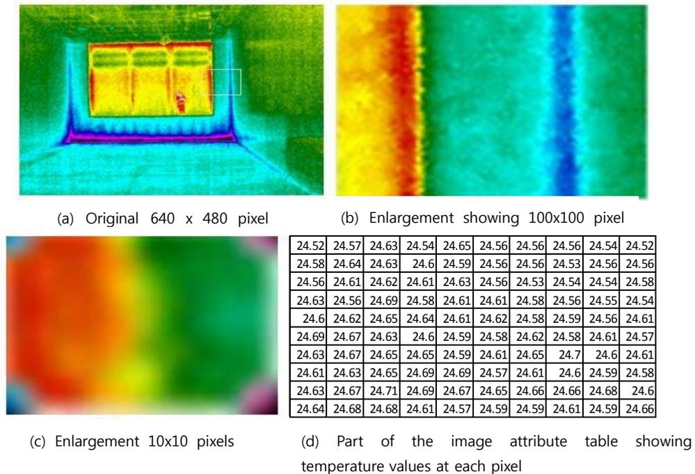
Fig. 7 Basic information of the thermal IR image
