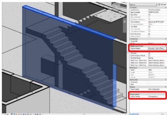
(c) Updated BIM showing concrete surface material and homogeneous texture of the interior walls
