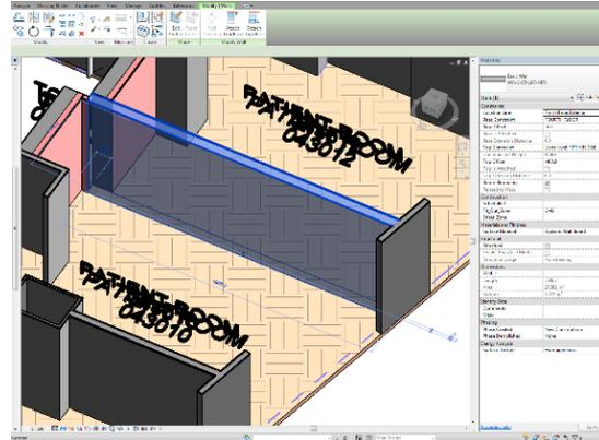
(b) Updated BIM showing Gypsum Wall Board material and homogeneous texture of the interior walls
