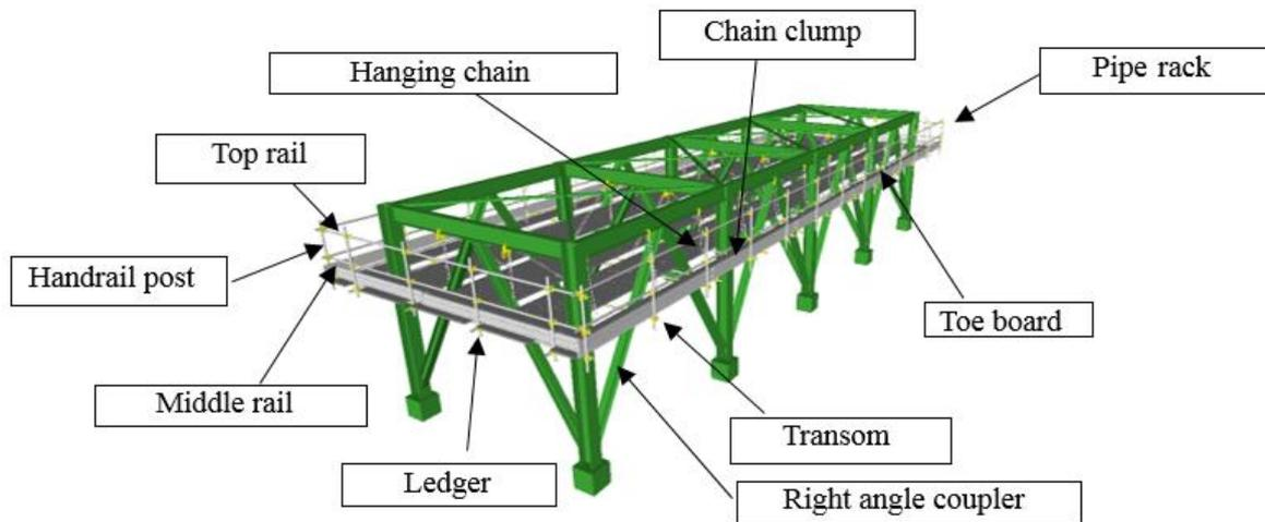
Fig. 4 Scaffold materials (Hara *et al.* 2018a)
