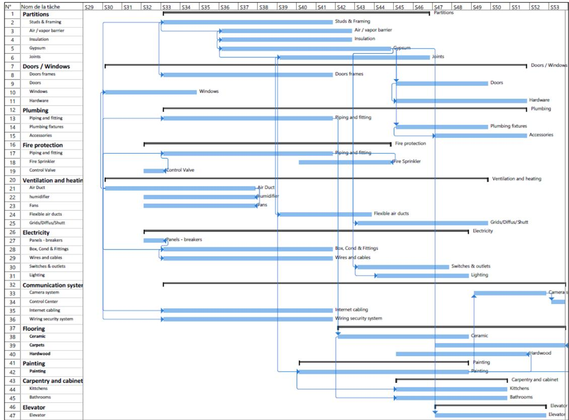
Fig. 1 Gantt-Precedence diagram scheduling for a building floor
