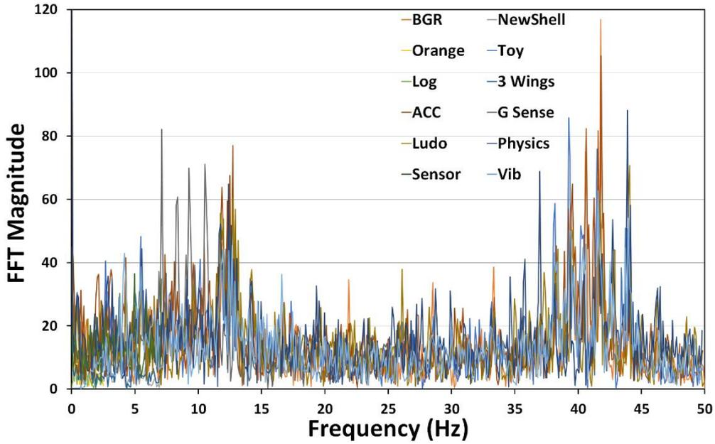
Fig. 8 Frequency response of each app under experimental excitation from simulated train-bridge interaction
