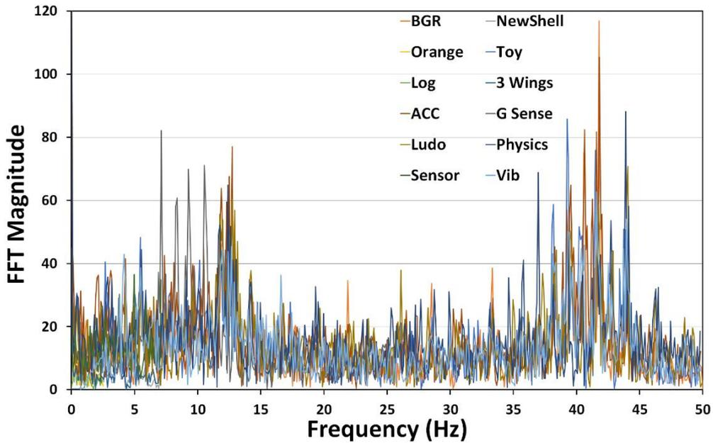
Fig. 9 Mean differences between individual App measurements and baseline accelerometer for TGV bridge passage
