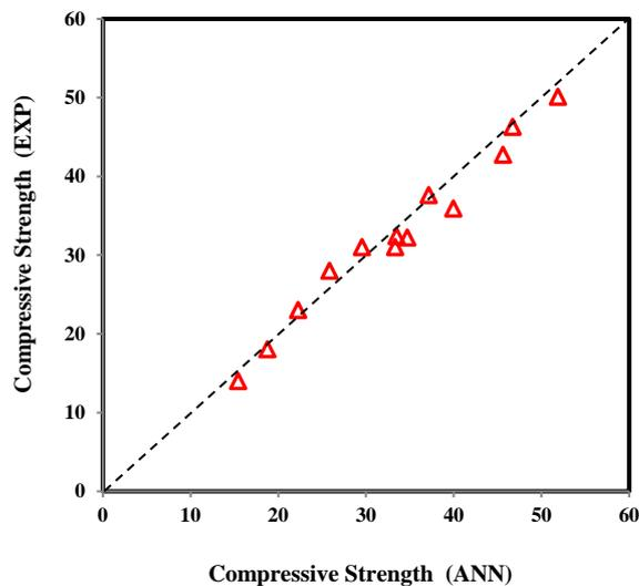
Fig. 5 Comparison between the ANN results and experimental results
