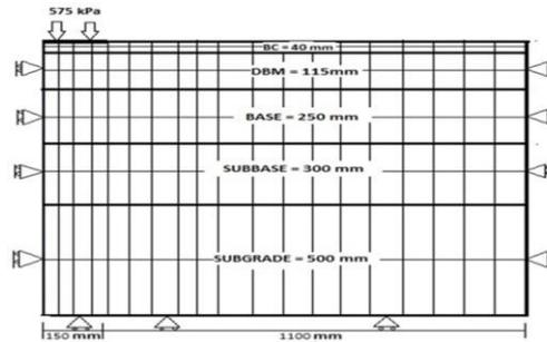
Fig. 2 Finite- element discretization of pavement section for unstabilized subgrade soil B
