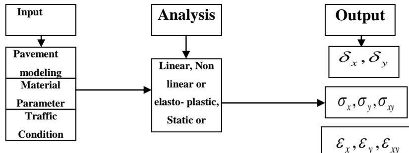
Fig. 1 System architecture for mechanistic approach
