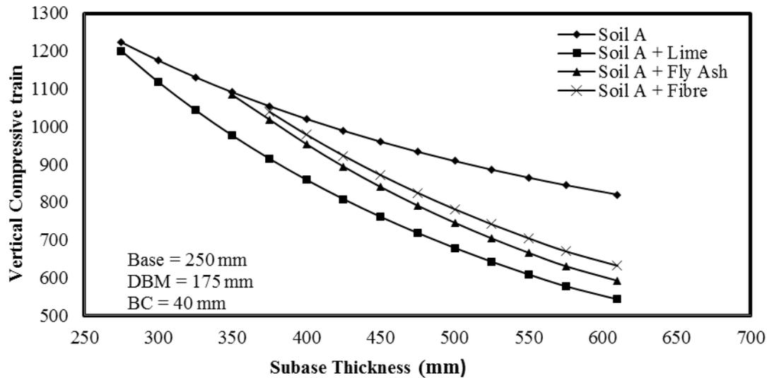
Fig. 3 Variation of vertical compressive strain at top of subgrade soil a with subbase thickness for pavement resting on unstabilized and stabilized subgrade
