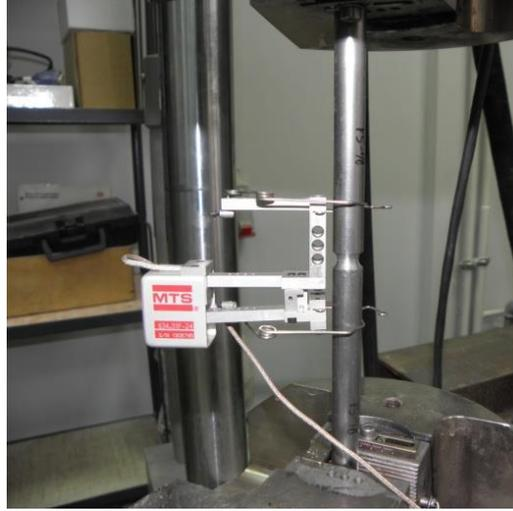
Fig. 3 An exemplary notched specimen under static tension
