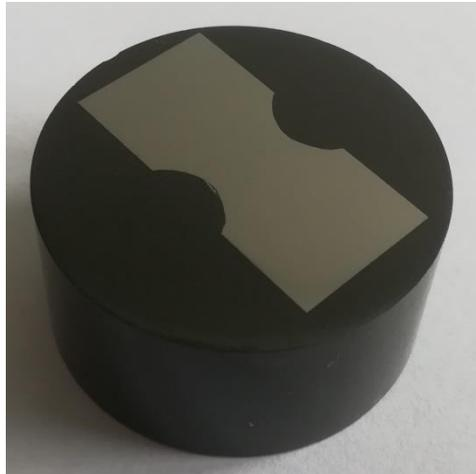
Fig. 7 An exemplary metallographic sample used to assess the structure of the steel
