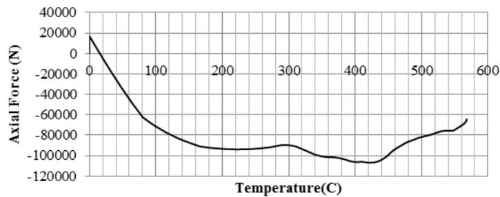
Fig. 23 Axial Force of at the center of slab A2-A3-B3-B2 at floor 10
