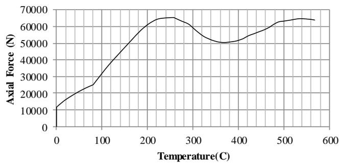
Fig. 21 Axial Force of at the center of slab A3-A4-B4-B3 at floor 10
