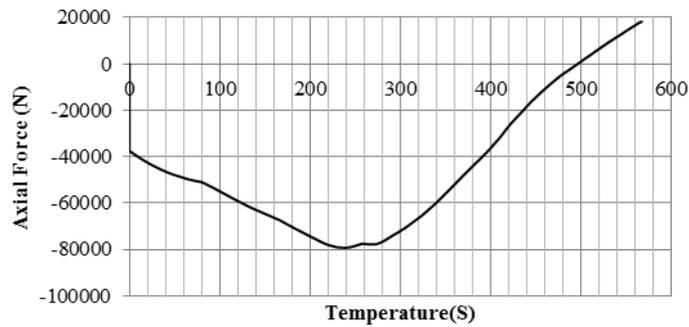
Fig. 22 Axial Force at the perimeter of slab A3-A4-B4-B3 at floor 10
