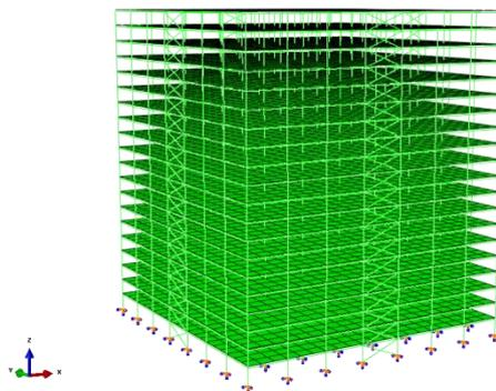
Fig. 1 3D Finite element model
