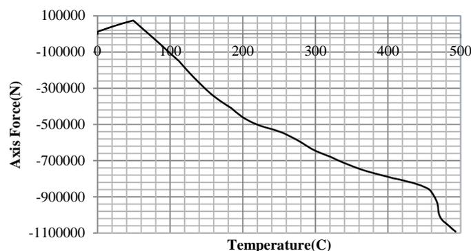
Fig. 6 Axial Force of Beam B1A1 at floor 10
