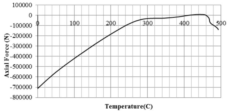
Fig. 11 Axial Force of Column A1 at floor 10
