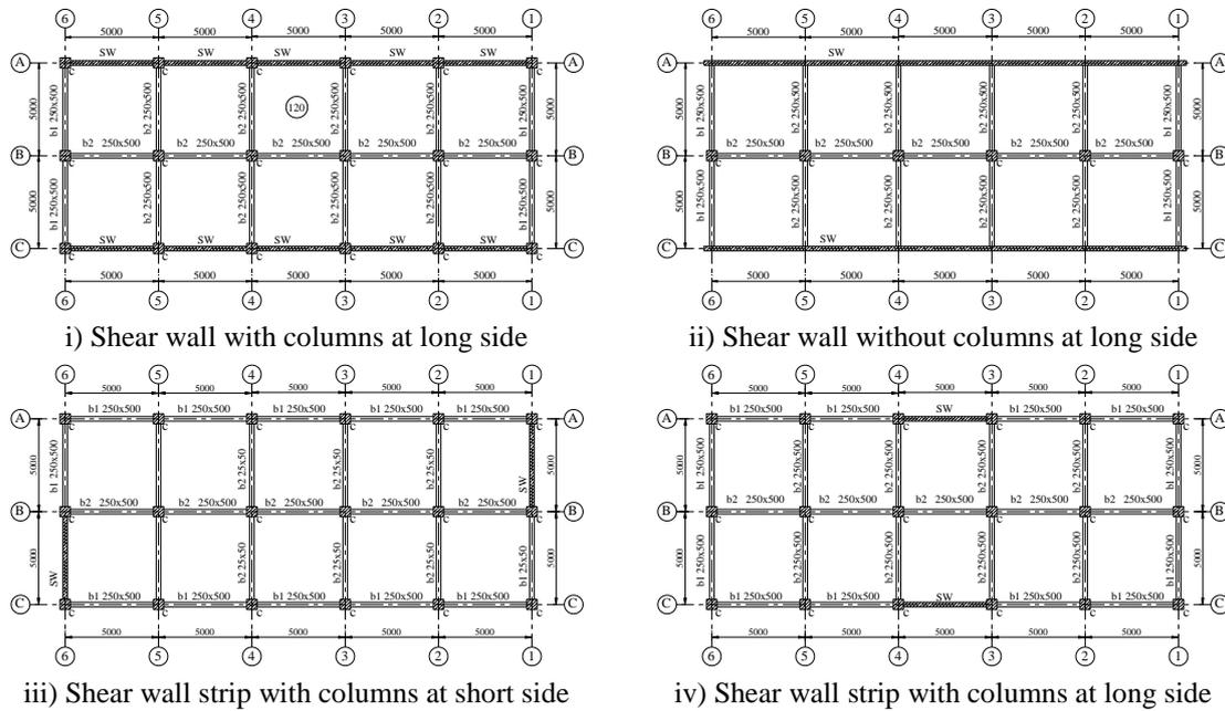
Fig. 2 Model (2) Rectangularity Ratio=2.5 (dimension in mm)
