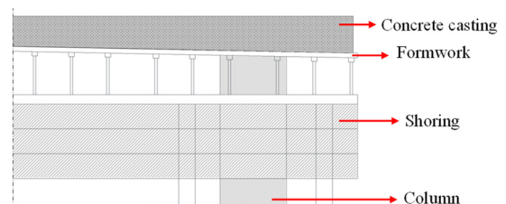
Fig. 7 On-site shoring system to support formwork
