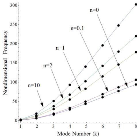
Fig. 14 Nondimensional frequency versus mode number containing different  $n$  value for clamped-free case (power law)
