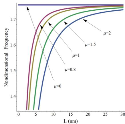
Fig. 12 Nondimensional frequency versus length with regard to different value for nonlocal parameter assumed for clamped-free FG nanobeam for sigmoid law
