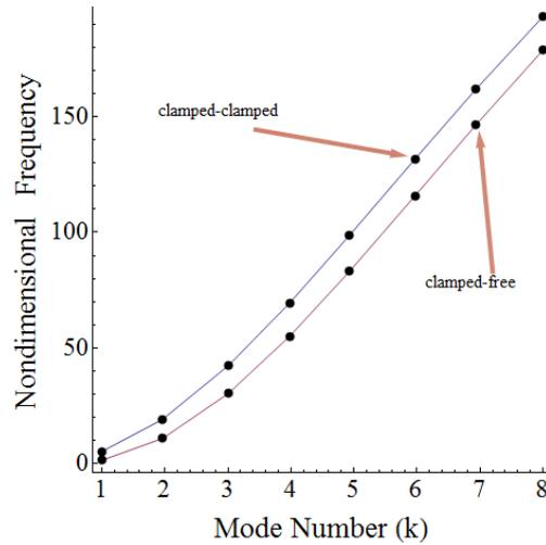
Fig. 15 Nondimensional frequency versus mode number for two boundary conditions demonstrated for exponential law
