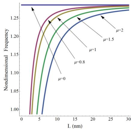
Fig. 11 Nondimensional frequency versus length with regard to different values for nonlocal parameter assumed for clamped-free FG nanobeam for exponential law
