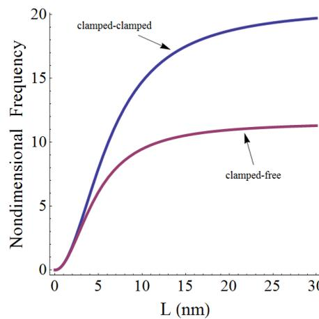
Fig. 18 Nondimensional frequency versus length for clamped-clamped and clamped-free conditions for exponential law ( $k=1$ )
