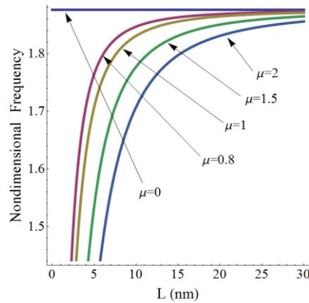
Fig. 10 Nondimensional frequency versus length with regard to different value for nonlocal parameter assumed for clamped-free FG nanobeam for power law
