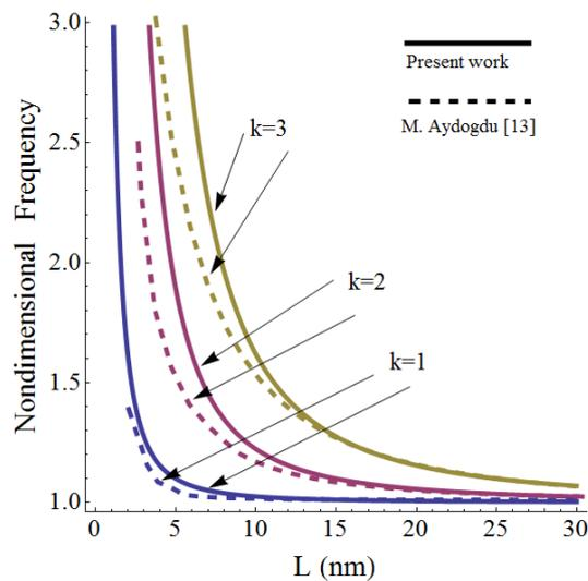
Fig. 3 Nondimensional frequency for clamped-free boundary condition
