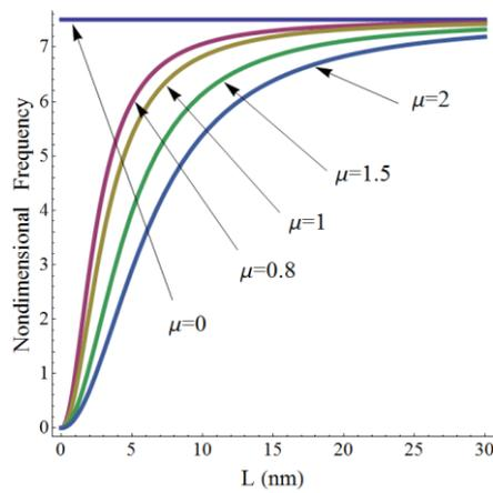
Fig. 7 Nondimensional frequency versus length with regard to different values for nonlocal parameter assumed for clamped-clamped FG nanobeam for power law
