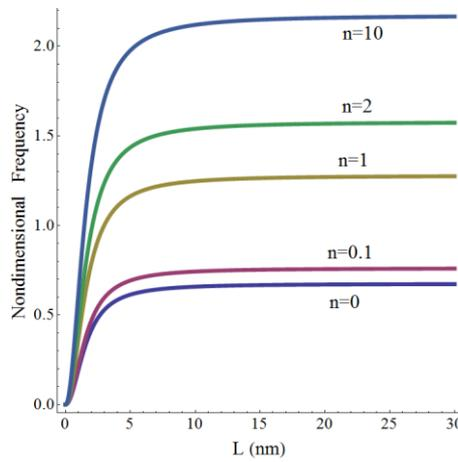
Fig. 17 Nondimensional frequency versus length for clamped-free boundary condition considering the 5 values for n parameter in power law function ( $k=1$  and  $\mu=1$  nm)
