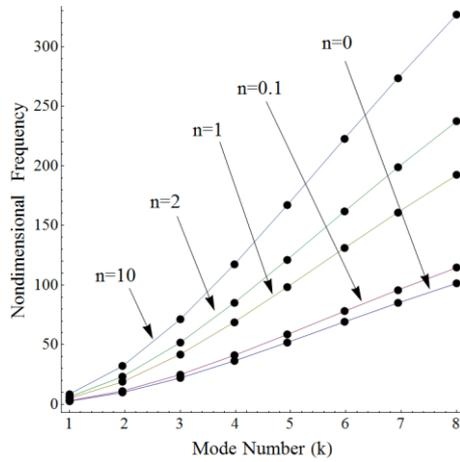
Fig. 13 Nondimensional frequency versus mode number containing different  $n$  value for clamped-clamped case (power law)
