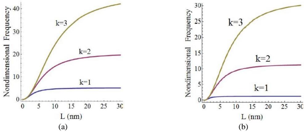
Fig. 5 Nondimensional frequency versus length for two boundary conditions containing (a) clamped-clamped and (b) clamped-free with the first three frequency modes for exponential law (nonlocal parameter 1 nm)
