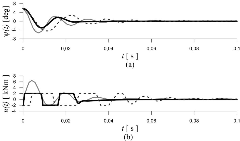
Fig. 11 Comparison of results obtained by MSAC (black), TPMT (grey) and fPID (dotted) controllers
