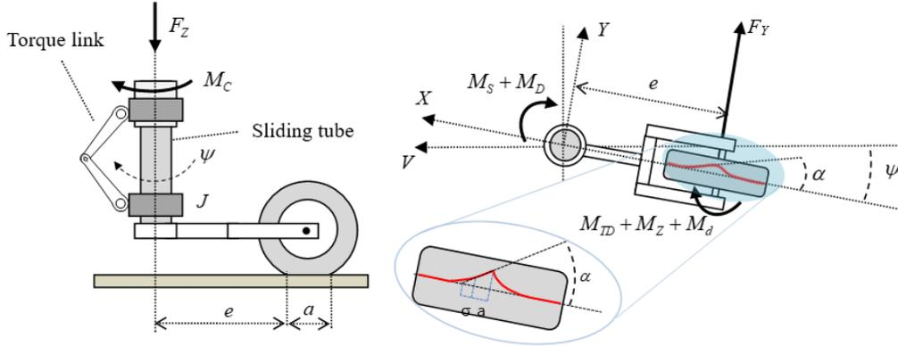
Fig. 2 Nose landing gear shimmy model
