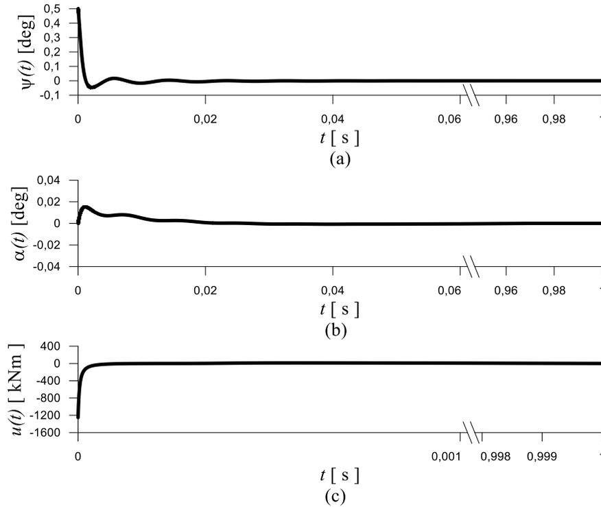
Fig. 7 Closed loop transient response without input saturation
