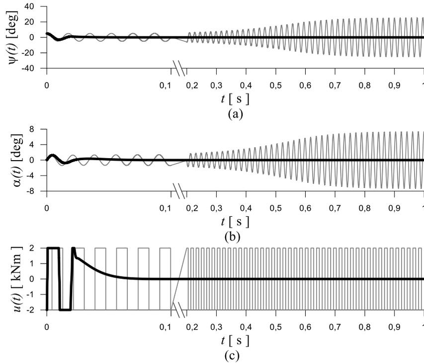
Fig. 9 Closed loop transient response with input saturation and anti-windup (black):  $V=30$  m/s,  $\psi_0=5$  deg
