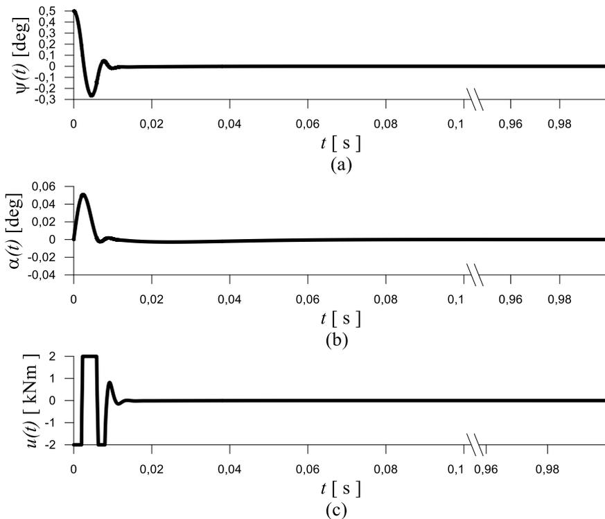
Fig. 8 Closed loop transient response with input saturation:  $V=20$  m/s,  $\psi_0=0.5$  deg
