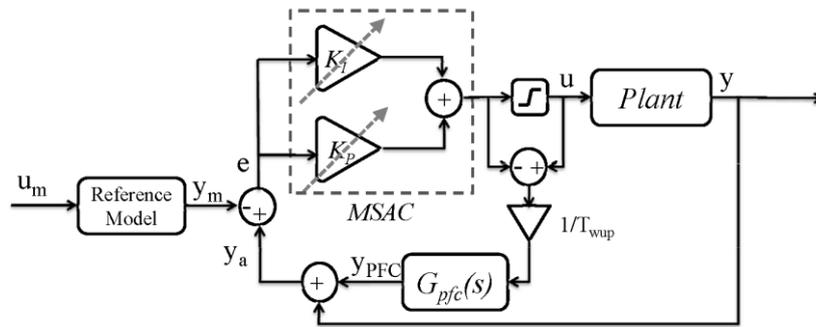
Fig. 10 PFC-MSAC scheme with saturation and Anti-Windup
