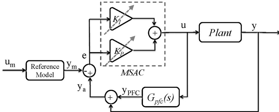
Fig. 1 Block diagram of PFC-MSAC controlled plant
