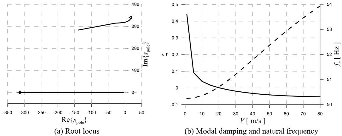
Fig. 4 System modal characteristics as function of speed
