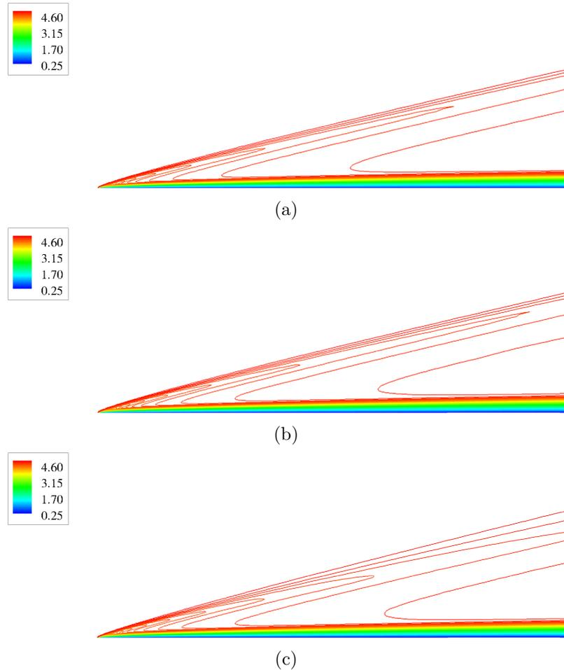
Fig. 9 Mach field in supersonic flow over a flat plate with FDS scheme (a), proposed hybrid scheme (b) and LLF scheme (c)
