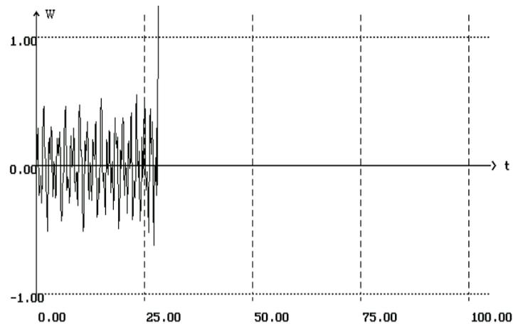
Fig. 2 Dependence of the deflection of the ideal-elastic plate on time  $t$  at  $V_{cr} = 1003$  m/s
