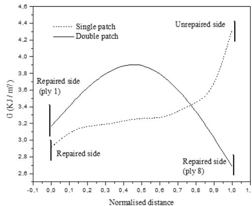
Fig. 17 Variation of the fracture energy in mixed mode along the crack front
