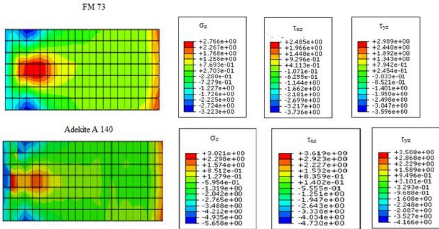
Fig. 13 Contour of peeling and shear stress in the adhesive layers
