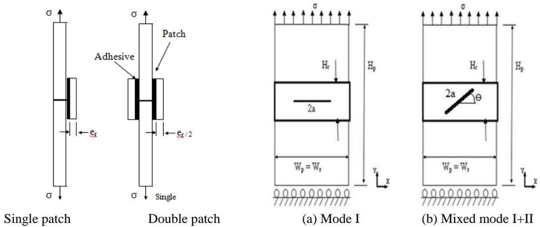
Fig. 1 Geometric model of plate with single and double patch for the pure mode I and mixed mode I+II
