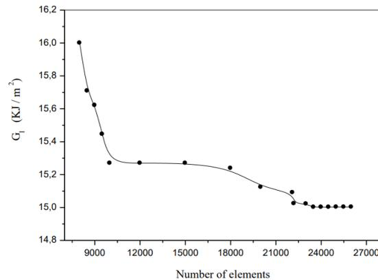
Fig. 4 Strain energy release rate Vs number of elements of cracked plate ( $a = 25$  mm)
