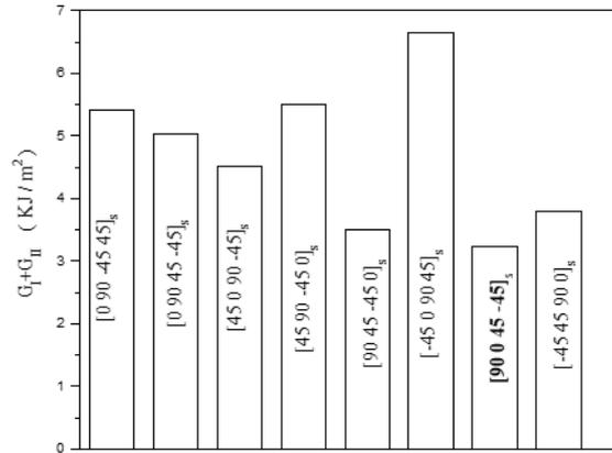
Fig. 18 Effect of plies orientation of the repaired plate on the GI+GII values ( $\theta = 45^\circ$ ,  $2a = 50$  mm)
