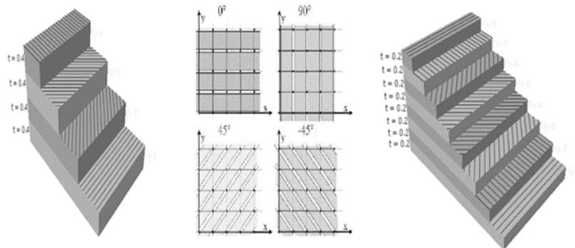
Fig. 3 Plies orientation in the patch and plate
