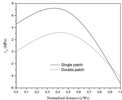
Fig. 15 Distribution of the shear stress  $\tau_{yz}$  along virtual line in adhesive layer
