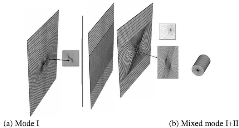
Fig. 2 Typical mesh model of the plate, patch and near the crack tip in pure mode I and mixed mode I+II
