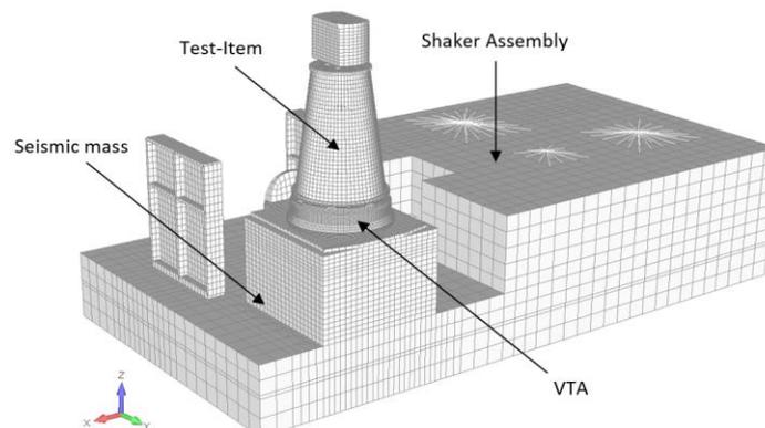
Fig. 5 Structure tested on the shaker, lateral configuration; excitation along Y
