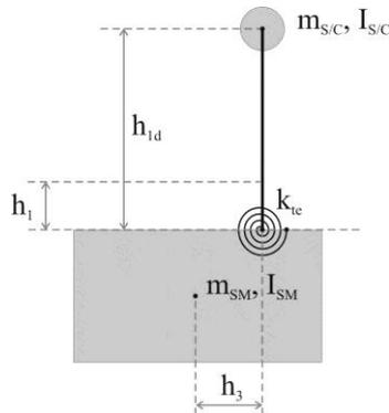
Fig. 1 Geometrical scheme and parameters of the system
