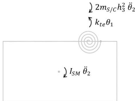
Fig. 3 Equilibrium of moments around the CoG of the seismic mass
