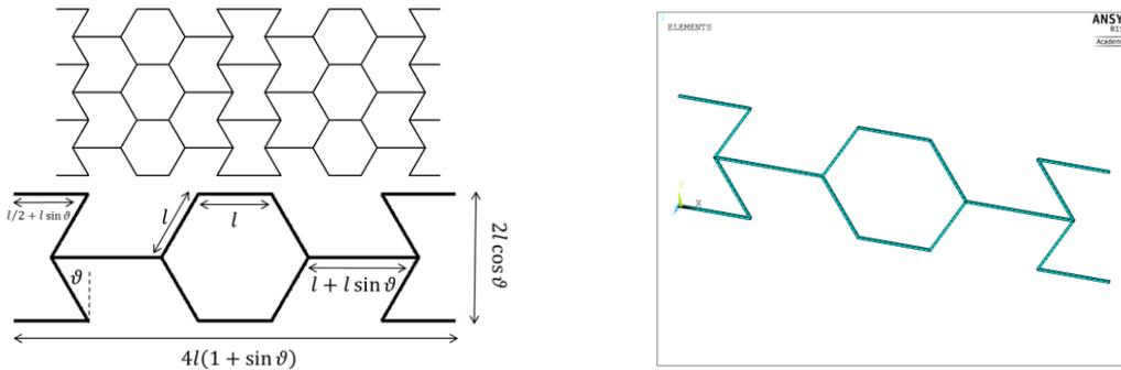
Fig. 10 AUXHEX unit cell (left) and example core (right)
