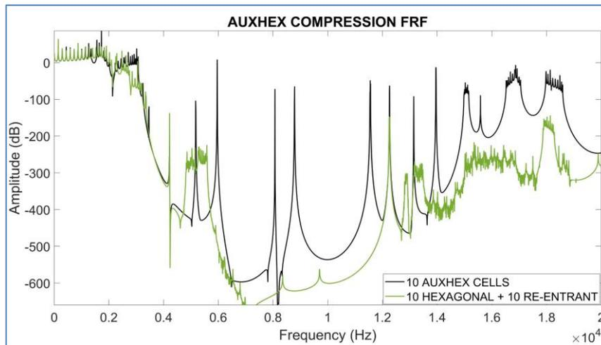
Fig. 21 Comparison between the output nodal solution at the end of the AUXHEX truss versus the output recorded at the end of the new truss (10 hexagonal + 10 re-entrant)
