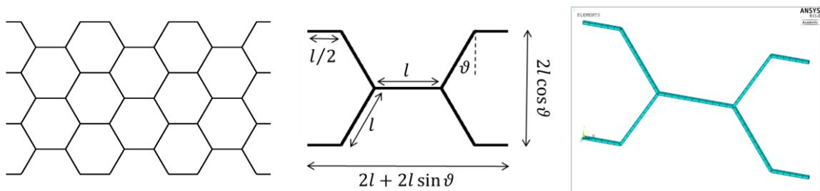
Fig. 4 Hexagonal unit cell (left) and example core (right)
