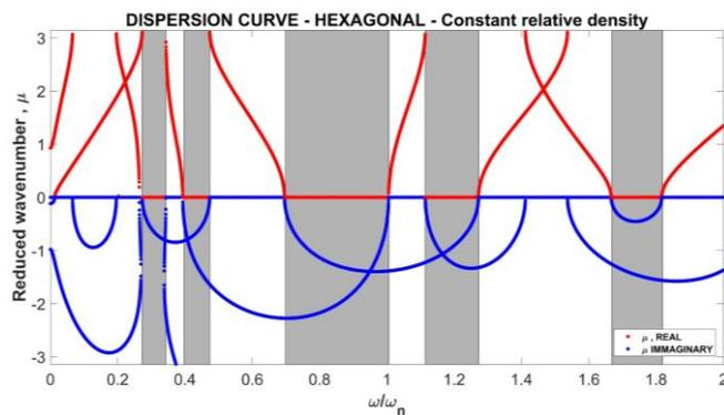
Fig. 6 Dispersion curve for Hexagonal topology
