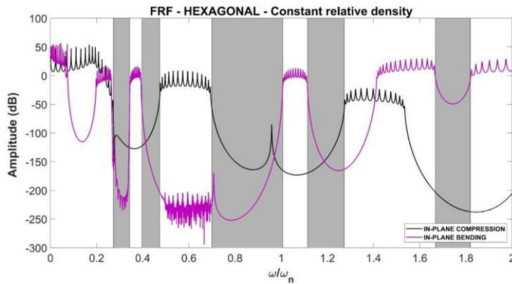
Fig. 5 FRF plot for Hexagonal topology
