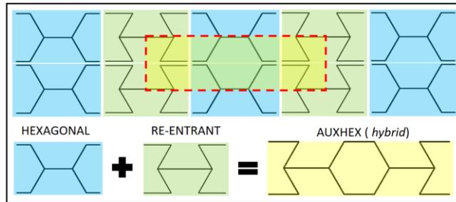
Fig. 16 Hybrid panel recreated with mixed unit cell (hexagonal and re-entrant) tessellation
