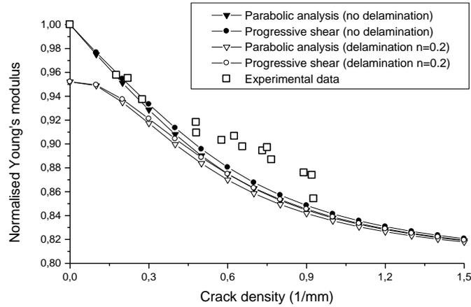
Fig. 3 Young's modulus reduction as function of crack density for T800H/3631 [0/90<sub>4</sub>]<sub>s</sub> laminate at room temperature
