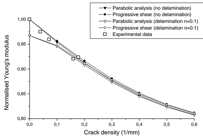
Fig. 7 Young's modulus reduction as function of crack density for T800H/3631  $[0/90_6]_s$  laminate at  $80^\circ\text{C}$
