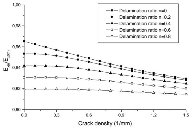
Fig. 13 The total stiffness degradation as a function of crack density for a  $[0/90]_{2s}$  glass/epoxy laminate with different delamination ratio ( $T=122^\circ\text{C}$ )
