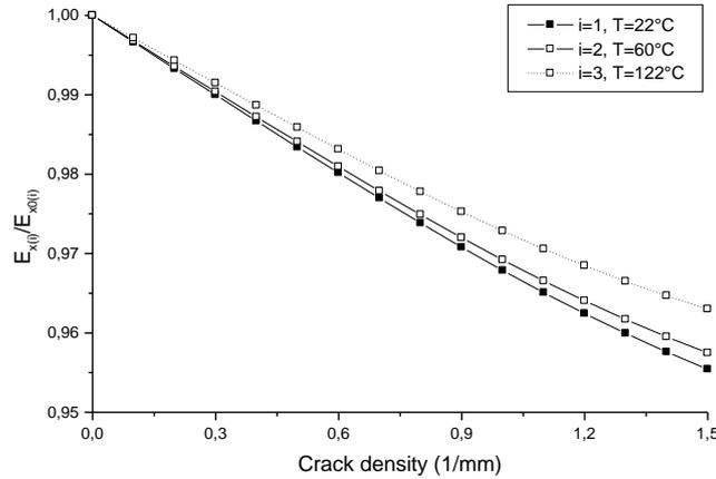
Fig. 9 Hygrothermal effect on the relative stiffness degradation due to: transverse cracks only in a  $[0/90]_{2s}$  glass/epoxy laminate
