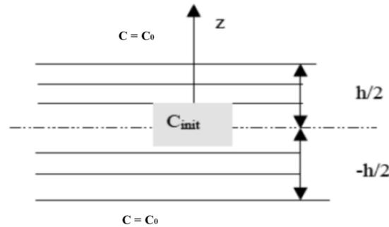
Fig. 8 The one-dimensional problem of moisture diffusion in plates
