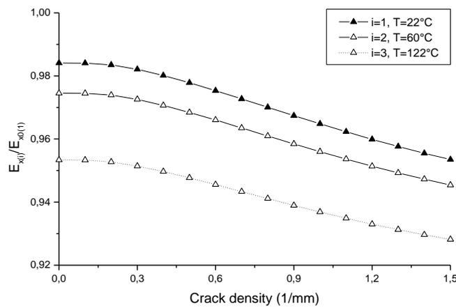
Fig. 12 Hygrothermal effect on the total stiffness degradation due to: transverse cracks and delamination in a  $[0/90]_{2s}$  glass/epoxy laminate ( $n=0.2$ )
