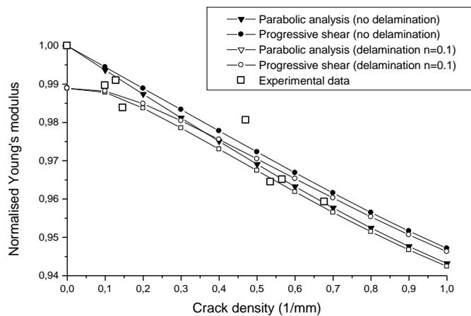
Fig. 5 Young's modulus reduction as function of crack density for T800H/3631 [0/90<sub>2</sub>]<sub>s</sub> laminate at 80°C
