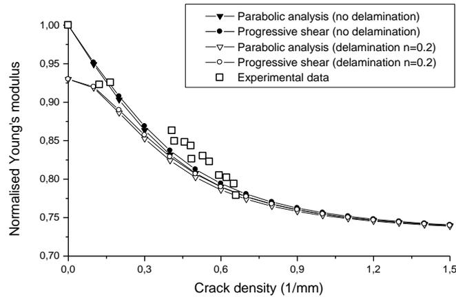
Fig. 4 Young's modulus reduction as function of crack density for T800H/3631 [0/90<sub>6</sub>]<sub>s</sub> laminate at room temperature
