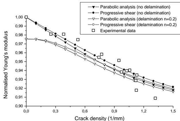
Fig. 2 Young's modulus reduction as function of crack density for T800H/3631  $[0/90_2]_s$  laminate at room temperature
