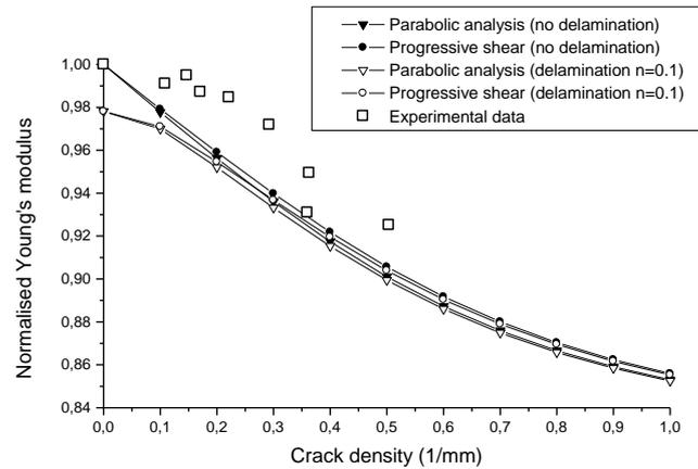
Fig. 6 Young's modulus reduction as function of crack density for T800H/3631  $[0/90_4]_s$  laminate at  $80^\circ\text{C}$
