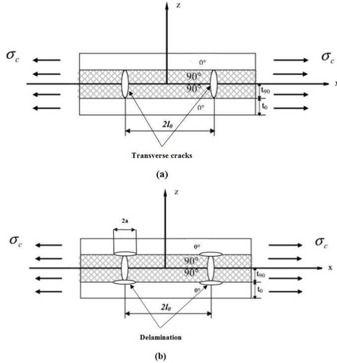
Fig. 1 Cross-ply composite laminates, (a) with transverse cracks and (b) with transverse cracks and delamination
