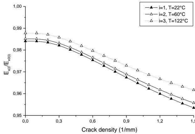
Fig. 10 Hygrothermal effect on the relative stiffness degradation due to: transverse cracks and delamination in a  $[0/90]_{2s}$  glass/epoxy laminate ( $n=0.2$ )
