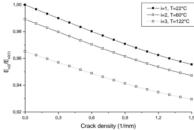
Fig. 11 Hygrothermal effect on the total stiffness degradation due to: transverse cracks only in a  $[0/90]_{2s}$  glass/epoxy laminate
