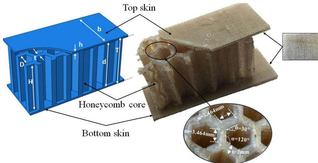
Fig. 5 CAD of honeycomb and sandwich structure
