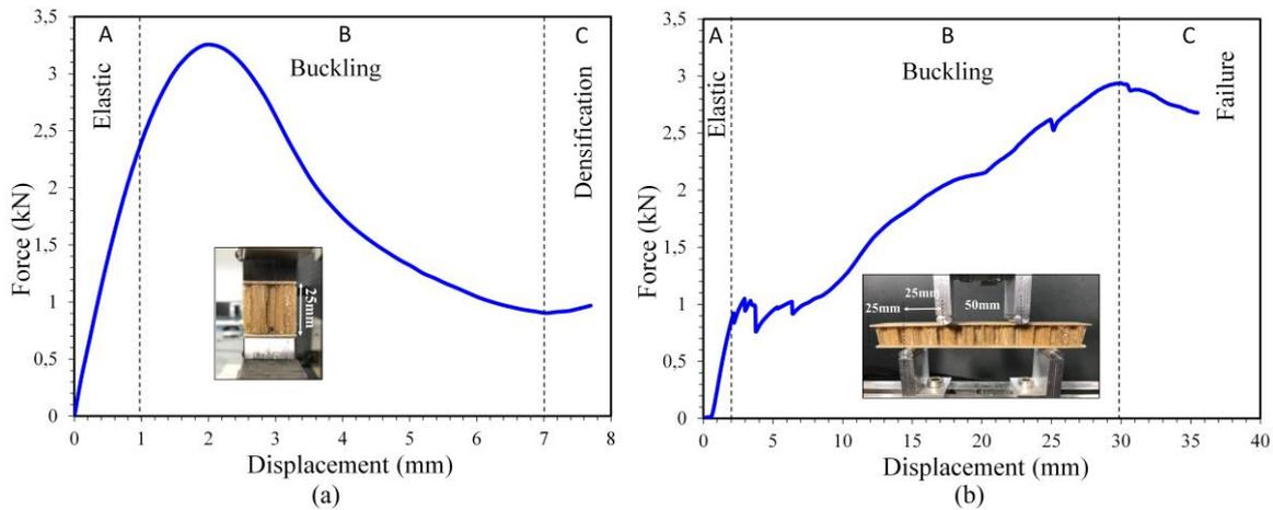
Fig. 6 Experimental force versus displacement (a) Compression test, (b) Flexural test
