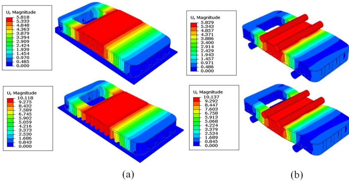
Fig. 17 Deformed cabin wall shaped honeycomb sandwich structure (a) Compression (b) Flexural
