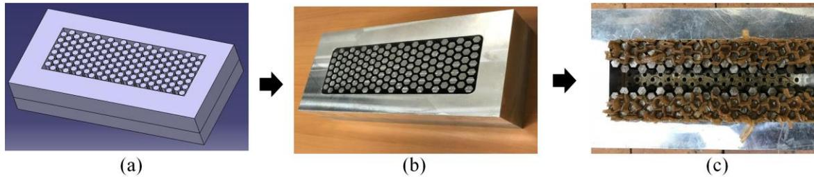
Fig. 3 Honeycomb mould: (a) CAD, (b) Mould, (c) Sandwich core fabrication
