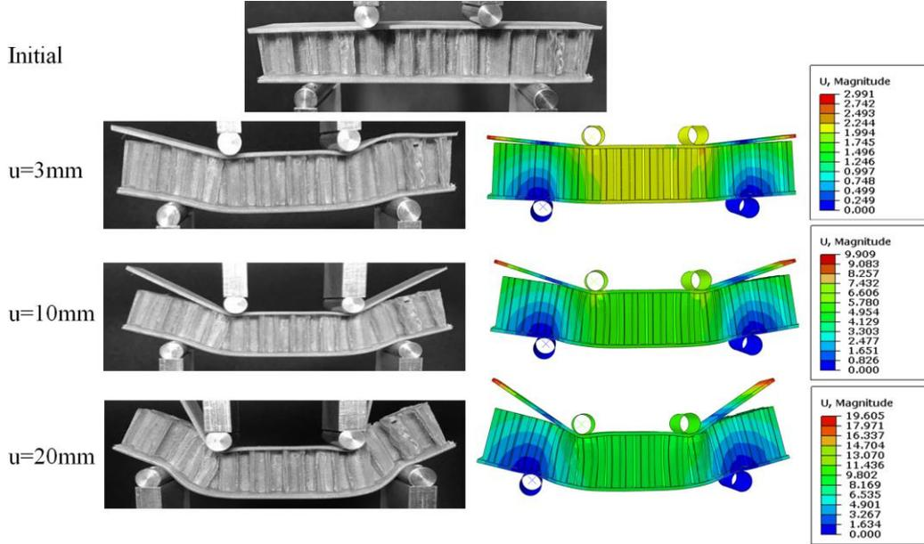
Fig. 9 Comparison of experimental and predicted 4-point deformed sandwich structure
