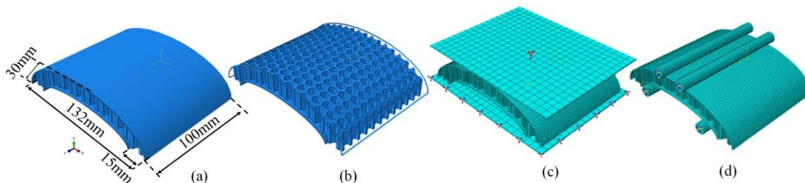
Fig. 10 Projectile shaped honeycomb (a) Geometry (b) Core (c) Compression (d) Flexural
