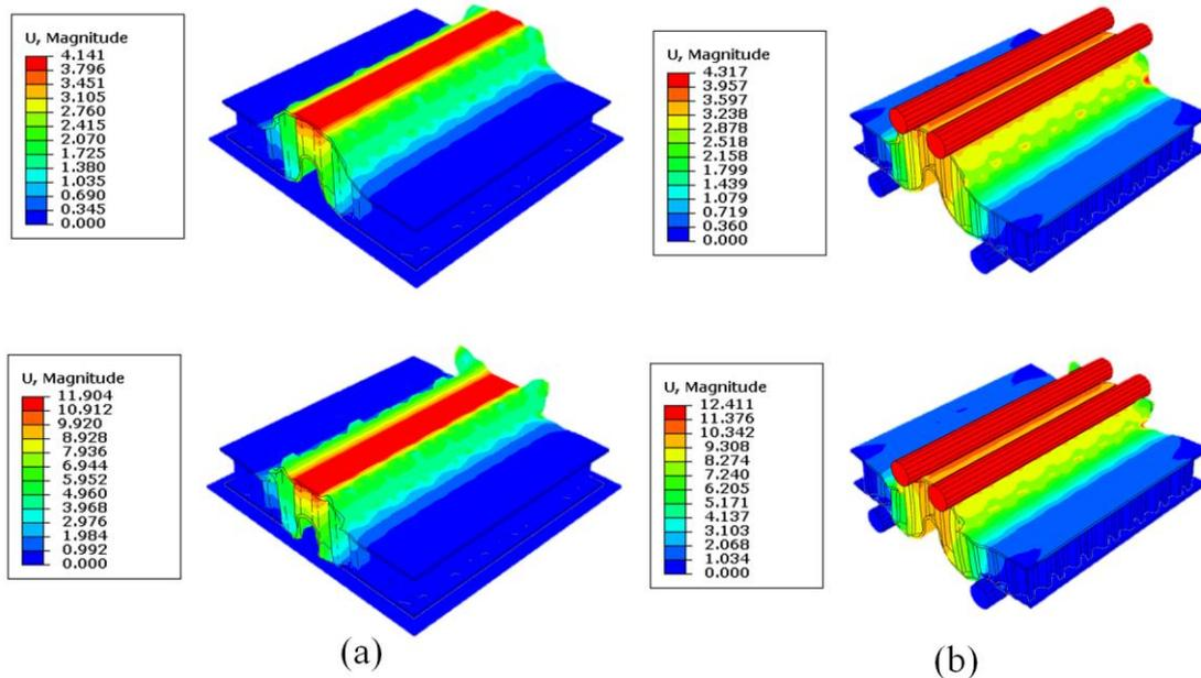
Fig. 15 Deformed dome shaped honeycomb (a) Compression (b) Flexural
