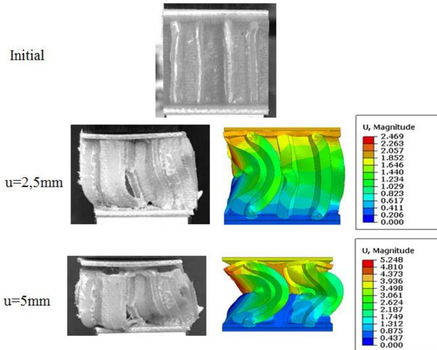
Fig. 8 Comparison of experimental and predicted compression deformed sandwich structure
