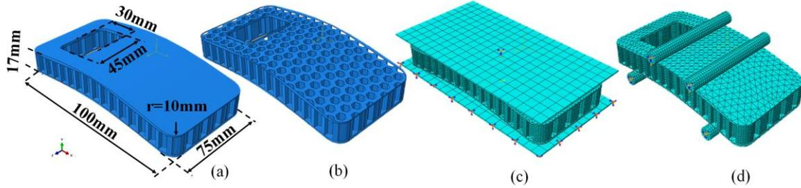
Fig. 16 Cabin wall shaped honeycomb (a) Geometry (b) Core (c) Compression (d) Flexural
