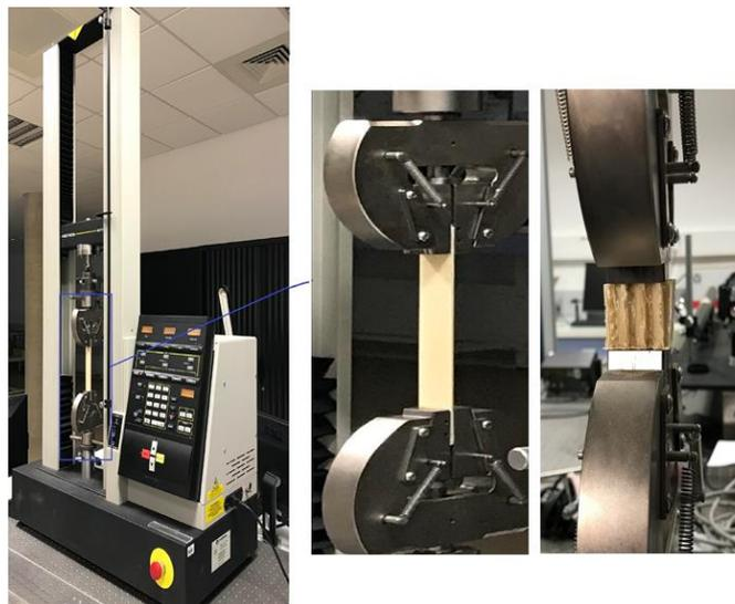
Fig. 4 Tensile and compression test setup for skin and core part
