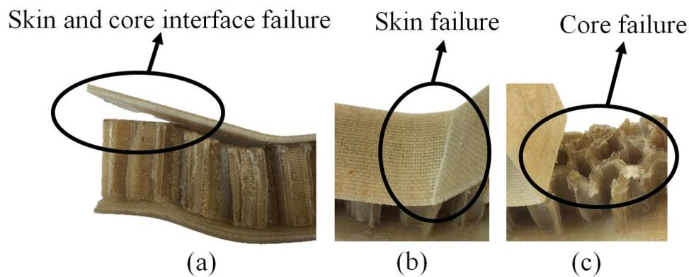
Fig. 7 Failure mechanisms (a) Skin/core interface failure, (b) Skin failure, (c) Core failure
