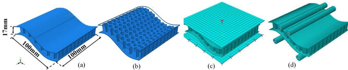
Fig. 12 Spline shaped honeycomb (a) Geometry (b) Core (c) Compression (d) Flexural
