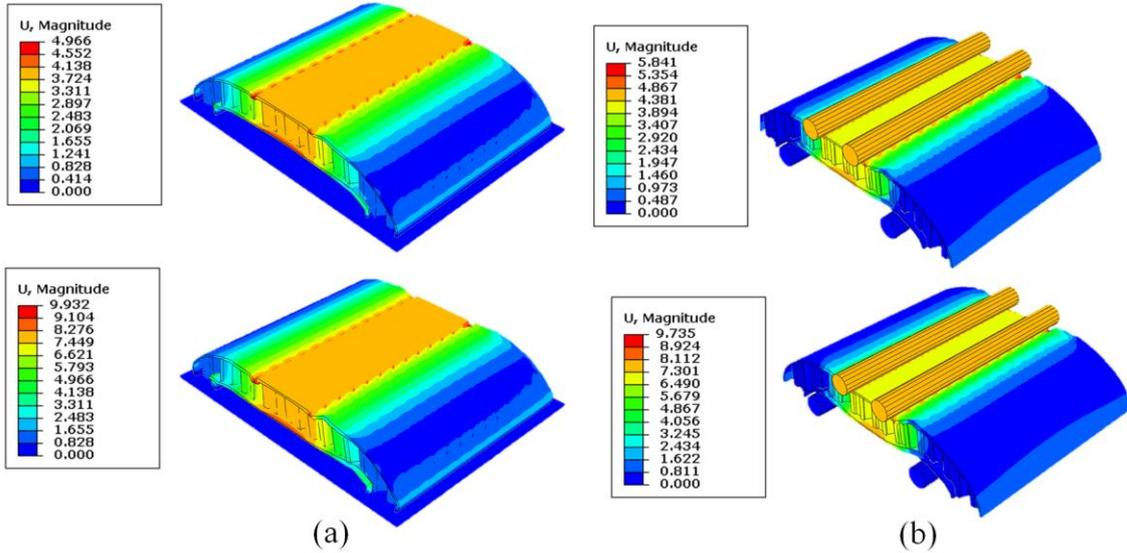
Fig. 11 Deformed projectile shaped honeycomb (a) Compression (b) Flexural
