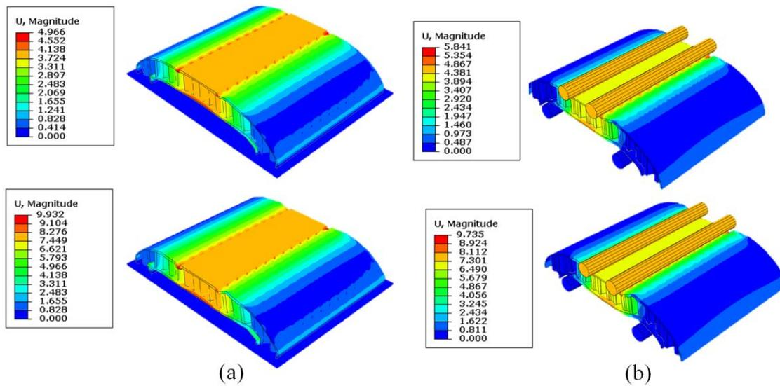
Fig. 13 Deformed spline shaped honeycomb (a) Compression (b) Flexural
