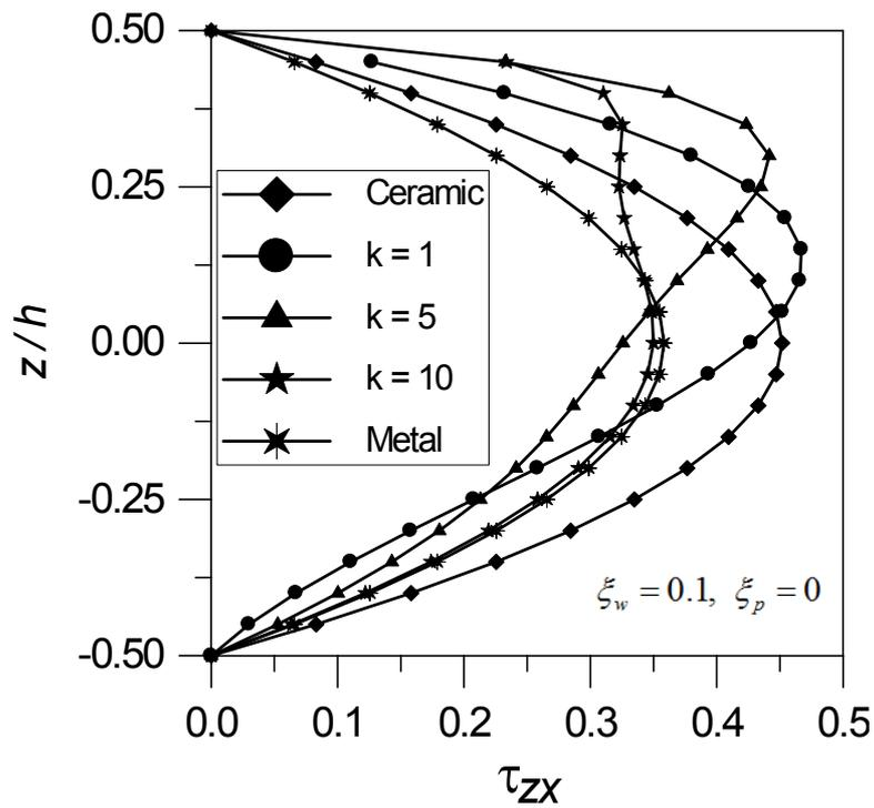
Fig. 10 Non-dimensional transverse shear stress through the thickness ( $L/h = 5$ )
