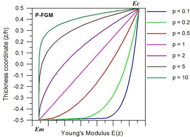
Fig. 2 Variation of Young's modulus  $E(z)$  through the thickness of FG beam for various values of the power-law index ( $p$ )
