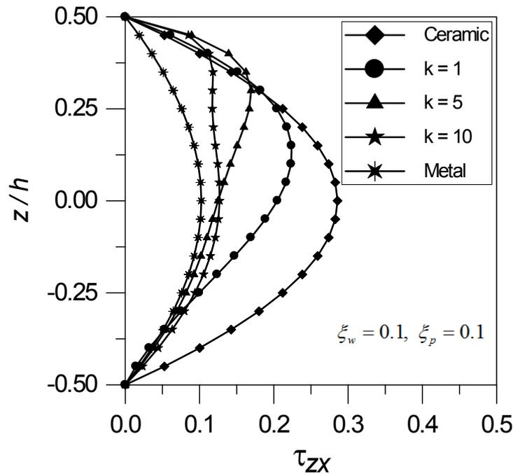
Fig. 11 Non-dimensional transverse shear stress through the thickness ( $L/h = 5$ )
