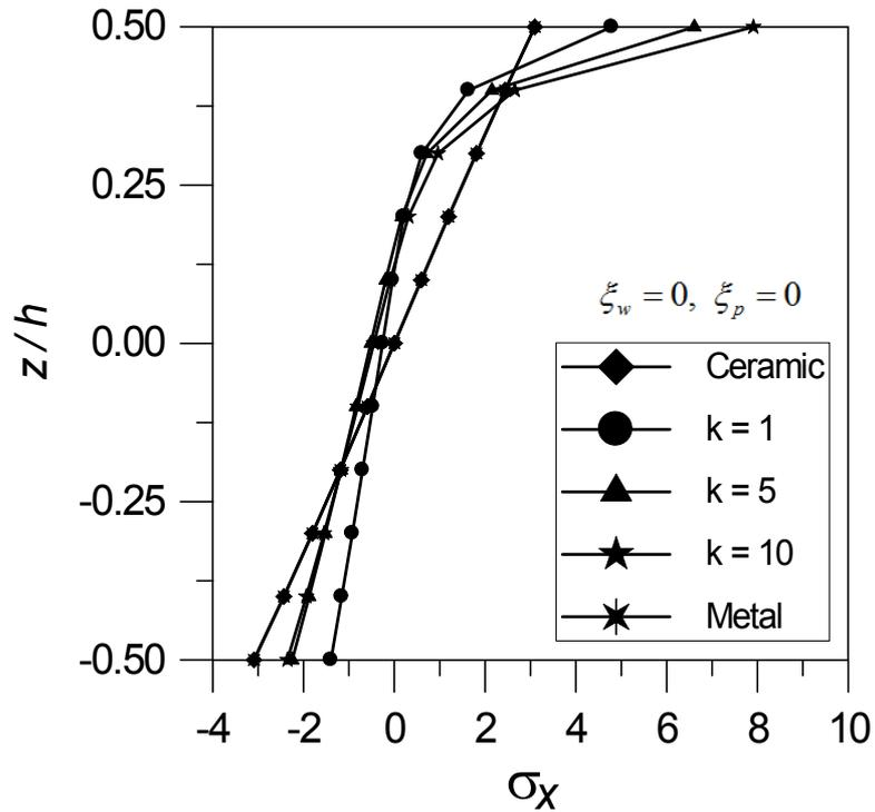
Fig. 6 Non-dimensional axial stress through the thickness ( $L/h = 5$ )
