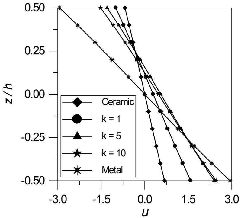
Fig. 4 Non-dimensional axial displacement through the thickness ( $L/h = 5$ )
