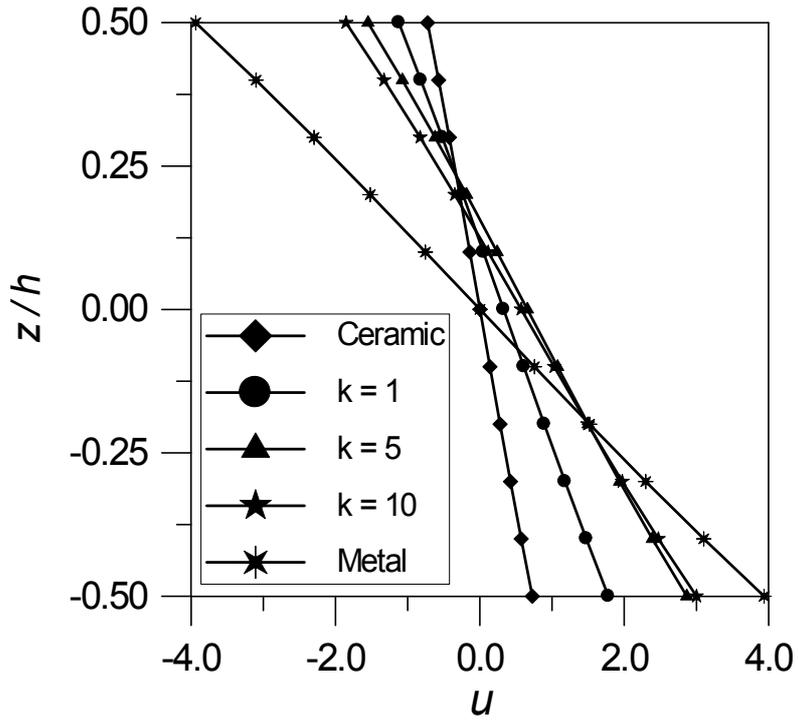
Fig. 3 Non-dimensional axial displacement through the thickness ( $L/h = 5$ )
