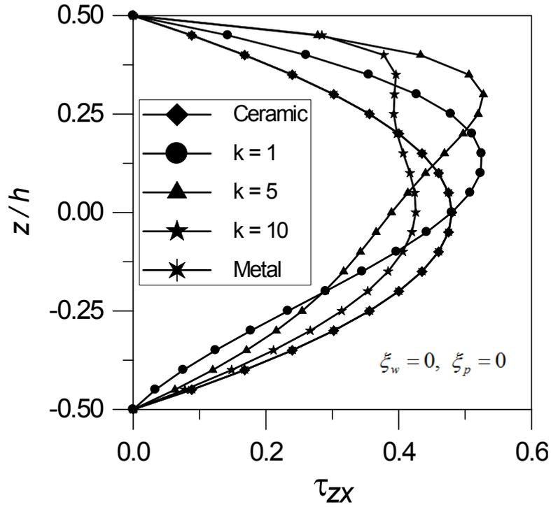
Fig. 9 Non-dimensional transverse shear stress through the thickness ( $L/h = 5$ )
