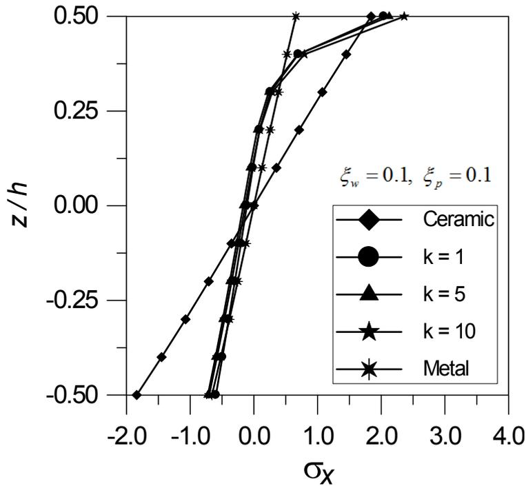
Fig. 8 Non-dimensional axial stress through the thickness ( $L/h = 5$ )
