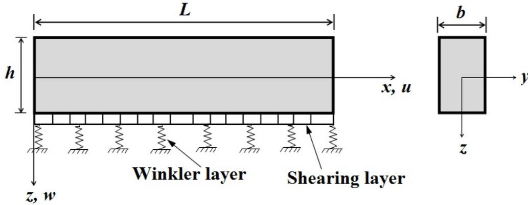
Fig. 1 FGM Beam resting on two parameter elastic foundation
