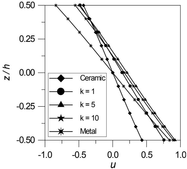
Fig. 5 Non-dimensional axial displacement through the thickness ( $L/h = 5$ )
