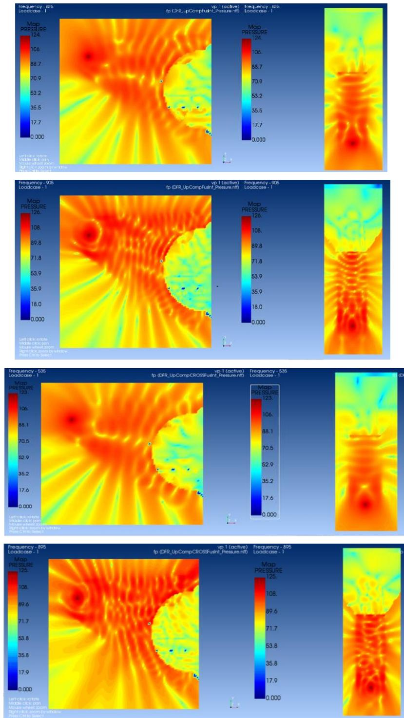
Fig. 12 Field maps of UFCI configuration at 625 Hz (first) and 905 Hz (second) and UFCCI configuration at 535 Hz (third) and 895 (fourth)
