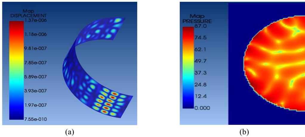
Fig. 6 NR – Cross-ply composite fuselage (UCFI) Displacement (left) and pressure (right) maps
