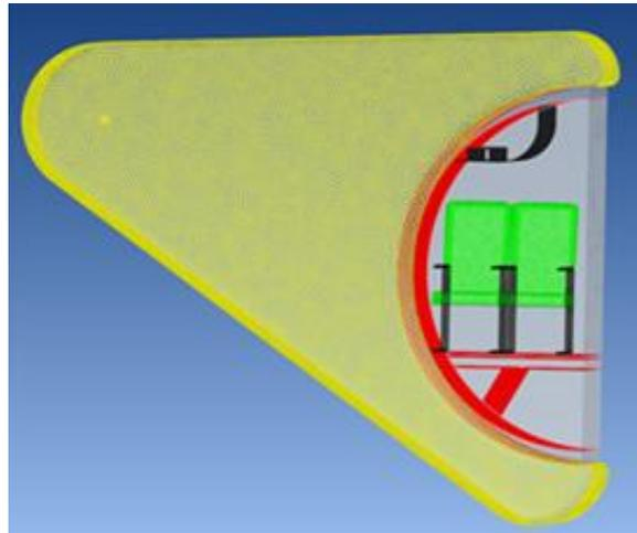
Fig. 7 Fuselage trunk with sound spherical source
