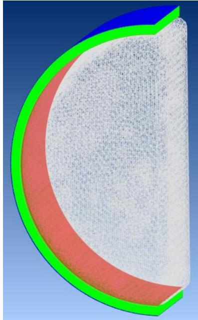
Fig. 4 Mesh of the semi-circular panel of the fuselage (stiffenings are included)
