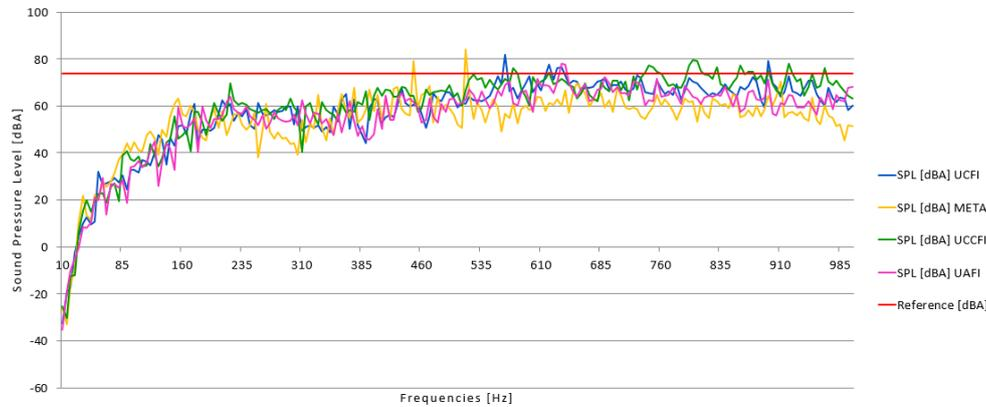
Fig. 15 Trend of sound pressure level at the head of the isle seat
