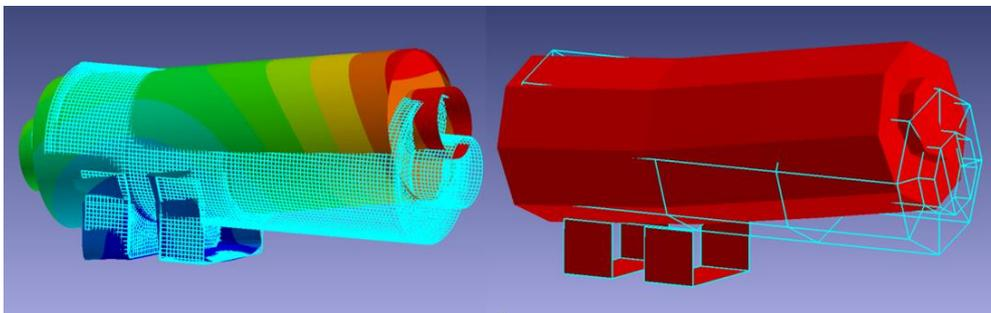
Fig. 6 Example comparison of the first mode shape between test and FEA results
