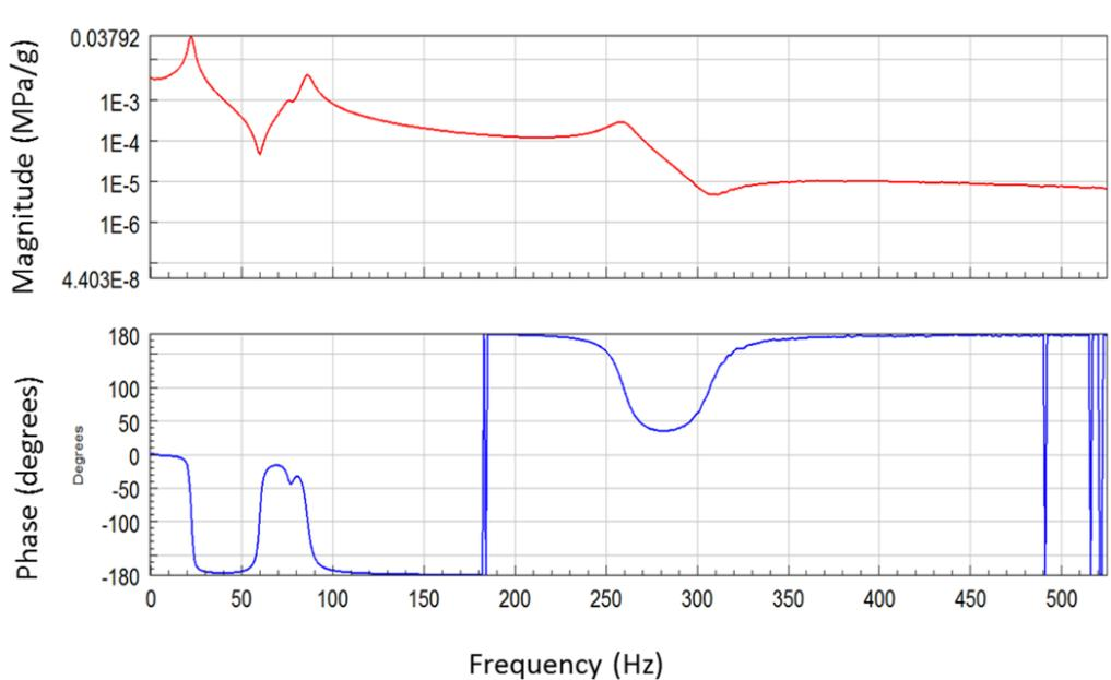
Fig. 4 Example Stress FRF obtained at a specific node
