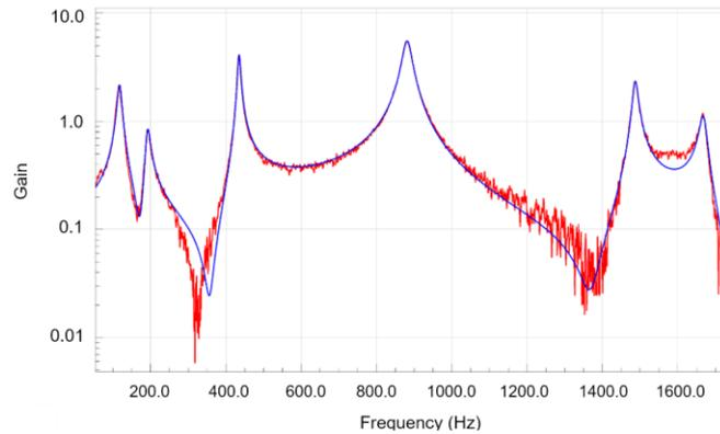
Fig. 7 Example curve fit of an FRF
