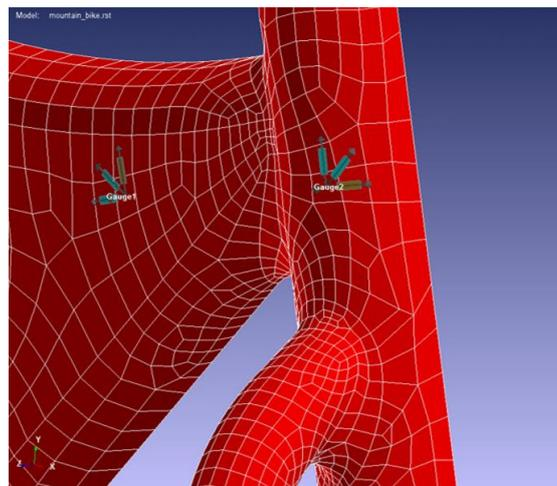
Fig. 8 Example use of virtual strain gages
