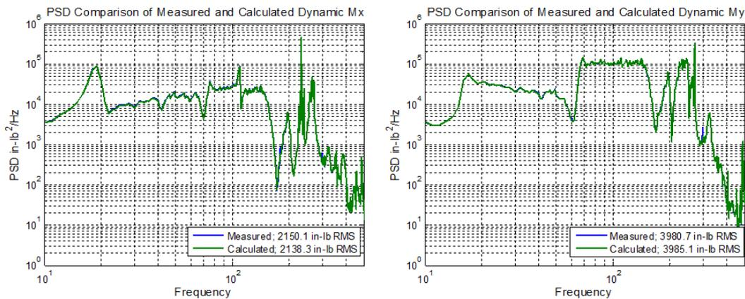
Fig. 9 Real-time moment limiting capability applied during spacecraft random vibration test (Van Dyke and Landry 2014)
