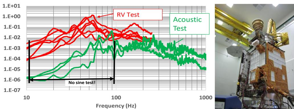
Fig. 2 Acceleration responses of a component measured at its interfaces on the SMAP Observatory that completed random vibration and acoustic testing are shown in this figure
