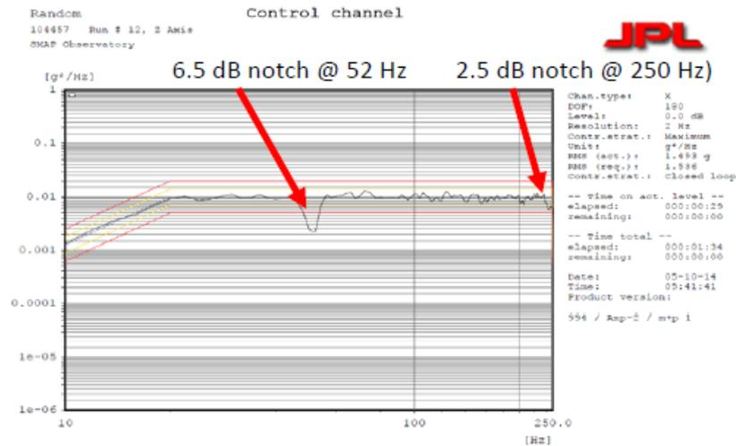
Fig. 8 Force-limited random vibration input to the SMAP Observatory that resulted in two notches: 6.5 dB @ 52 Hz and 2.5 dB @ 250 Hz
