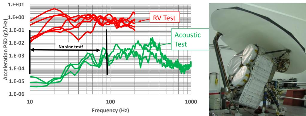
Fig. 1 Acceleration responses of a component measured at its interfaces on the Aquarius Instrument that completed random vibration and acoustic testing are shown in this figure
