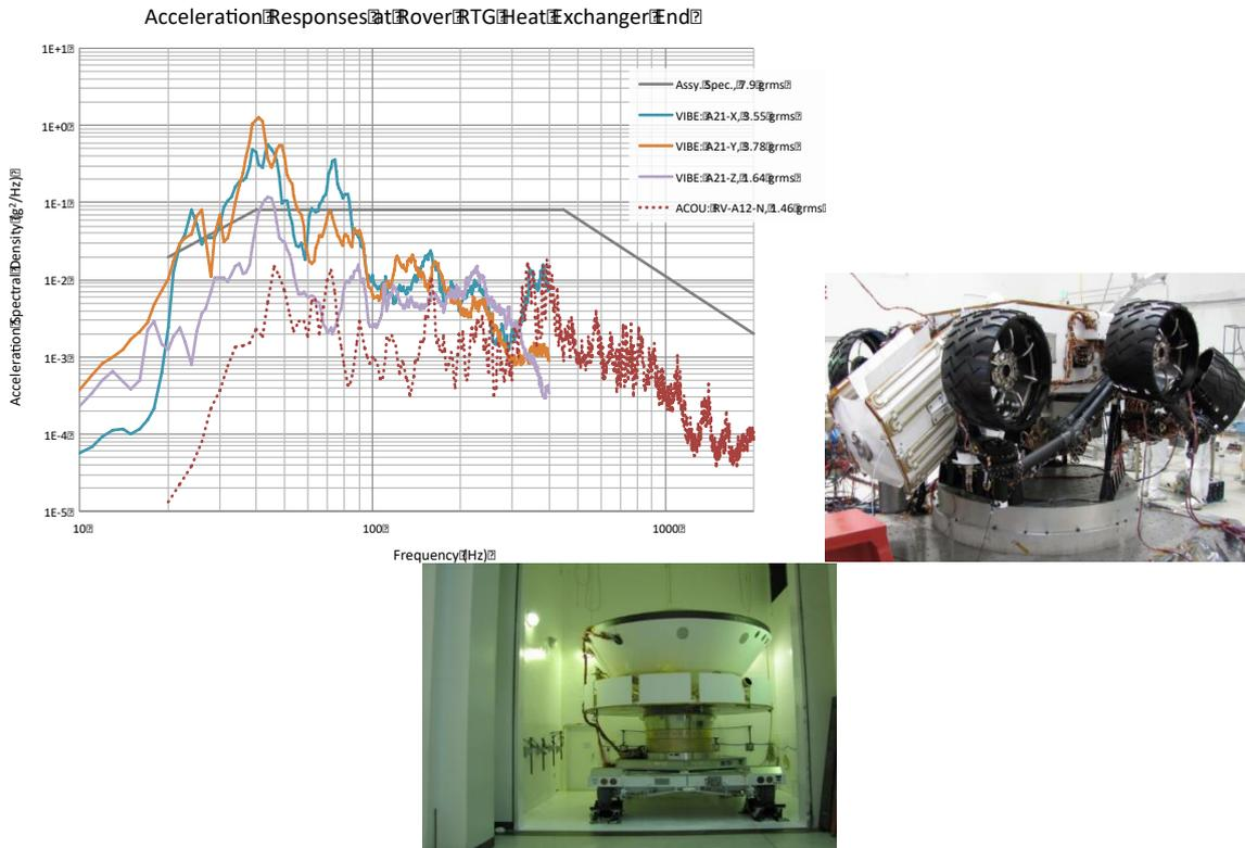
Fig. 3 A third example of a spacecraft (MSL) that successfully completed random vibration and acoustic testing. Acceleration responses from a component on the Rover are shown in this figure
