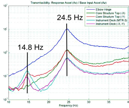
Fig. 4 Transmissibilities obtained from the SMAP Observatory vertical axis RV test indicating the presence of x-bending modes at 14.8 Hz and 24.5 Hz
