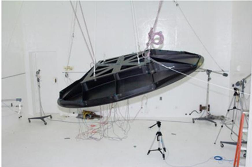
Fig. 7 Aquarius Reflector suspended in the acoustic chamber
