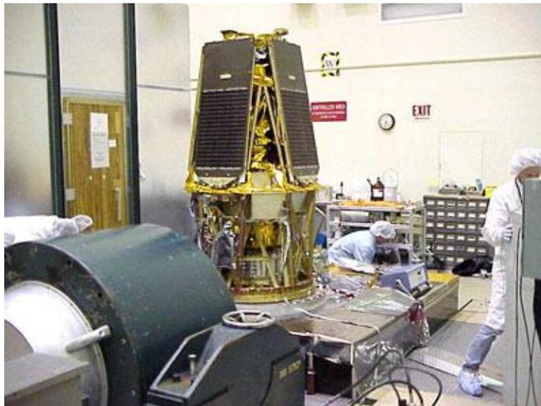
Fig. 6 HESSI Instrument test configuration on vibration shaker
