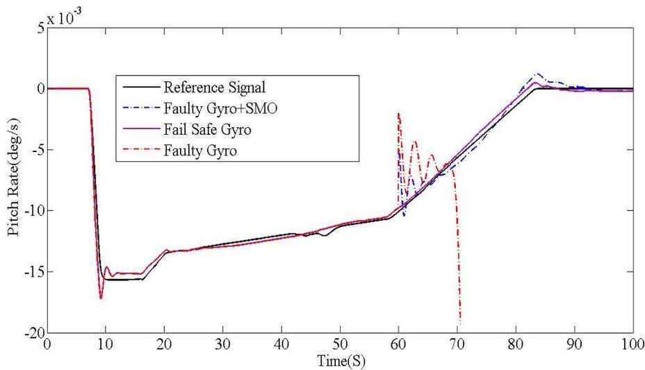
Fig. 6 Performance of the proposed fault recovery strategy at  $t=60$  s
