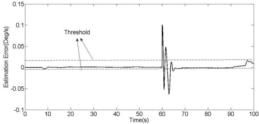
Fig. 5 Gyro fault detection in the presence of bias fault at  $t=60$  s
