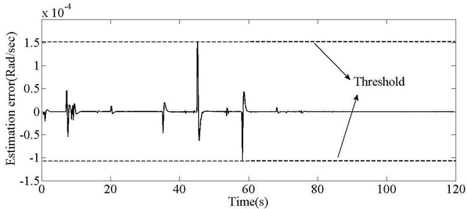
Fig. 4 The residual(estimation error) in a fault-free case obtained by SMO
