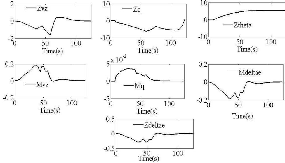
Fig. 1 Variation in dynamic coefficients of Pitch channel
