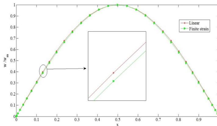
Fig. 10 Deflection of the first mode of the simply-simply supported carbon/epoxy composite beam
