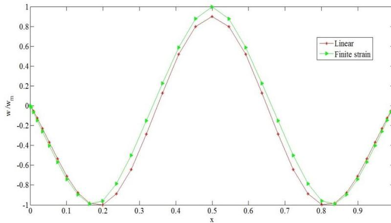
Fig. 9 Deflection of the third mode of the clamp-clamp supported glass/epoxy composite beam
