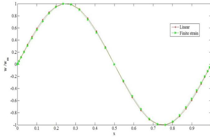
Fig. 11 Deflection of the second mode of the simply-simply supported carbon/epoxy composite beam
