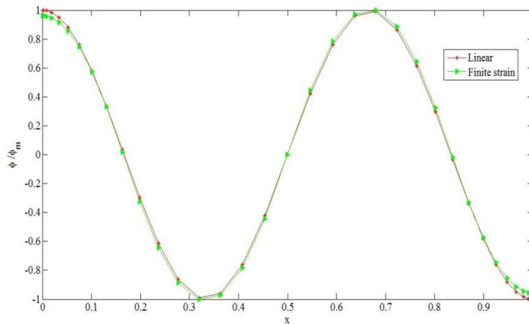
Fig. 15 Cross section rotation of the third mode of the simply-simply supported carbon/epoxy composite beam
