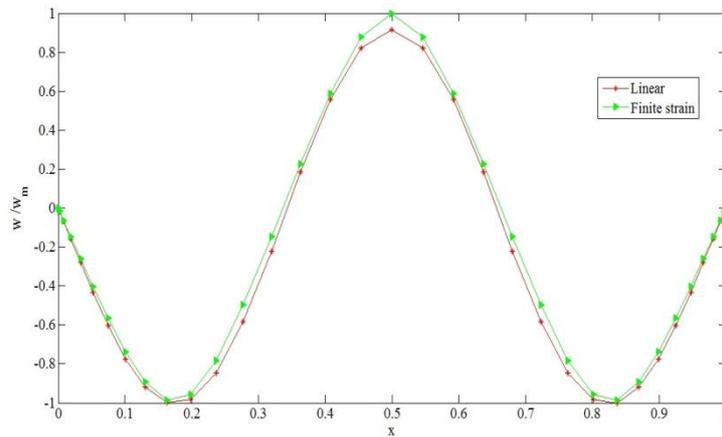
Fig. 3 Deflection of the third mode of the clamp-clamp supported carbon/epoxy composite beam
