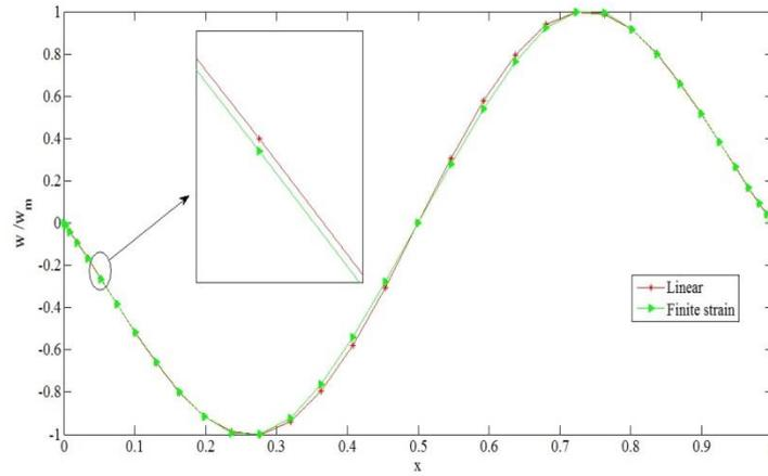
Fig. 2 Deflection of the second mode of the clamp-clamp supported carbon/epoxy composite beam
