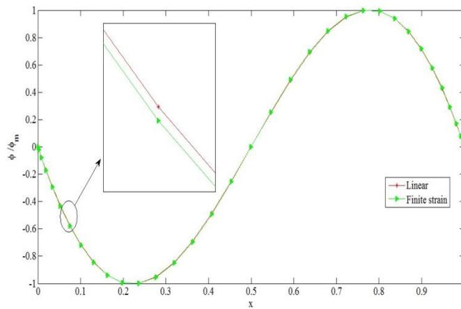
Fig. 4 Cross section rotation of the first mode of the clamp-clamp supported carbon/epoxy composite beam
