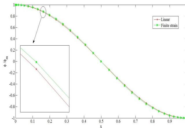
Fig. 13 Cross section rotation of the first mode of the simply-simply supported carbon/epoxy composite beam
