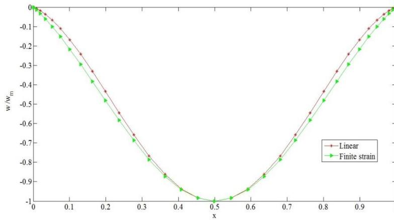
Fig. 7 Deflection of the first mode of the clamp-clamp supported glass/epoxy composite beam
