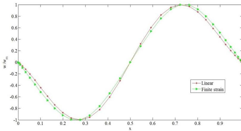
Fig. 8 Deflection of the second mode of the clamp-clamp supported glass/epoxy composite beam
