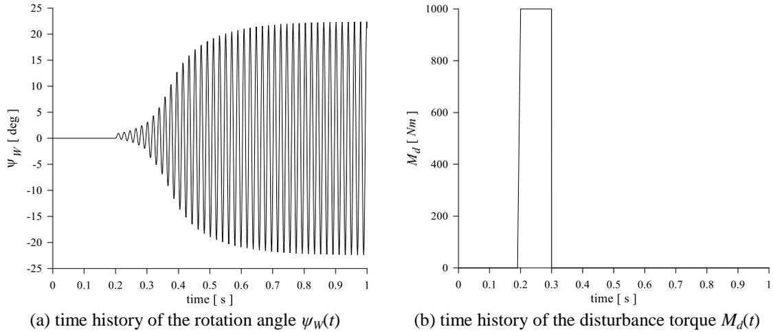
Fig. 2 Tire damage case: open loop results
