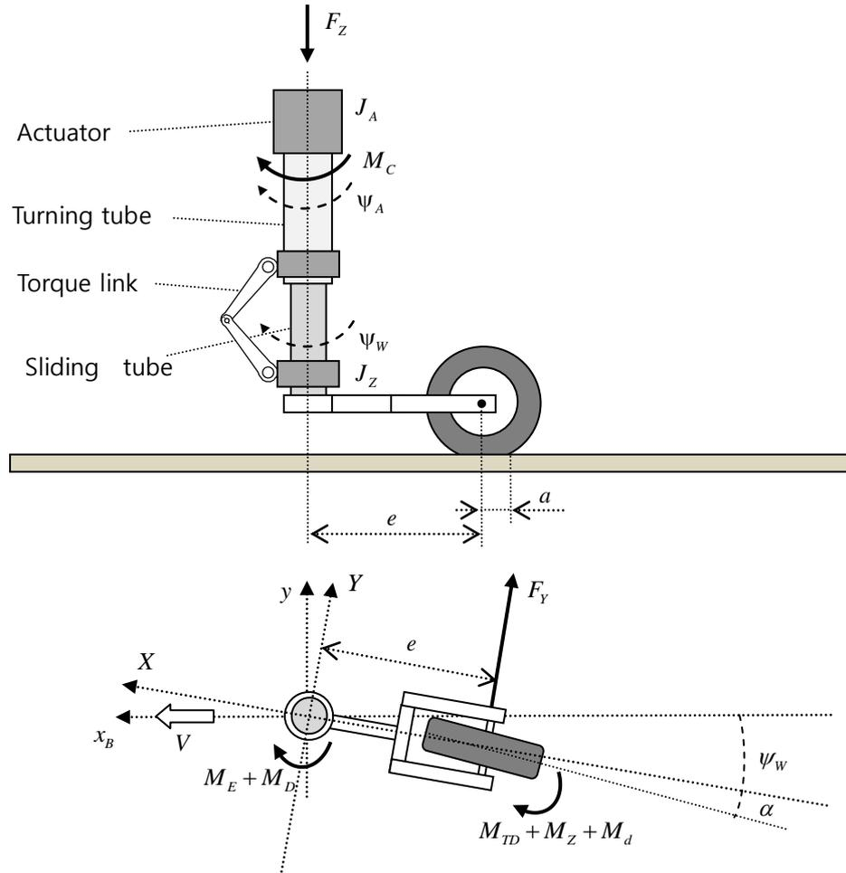
Fig. 1 Model of the nose landing gear
