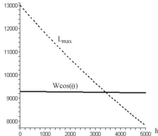
Fig. 3  $W\cos(\theta)$ , represented by the solid line, and  $L_{\max}$ , represented by the dotted line, as a function of the altitude, for the climbing airplane CP-1 at  $20^\circ$ , with a constant speed of 25 m/s
