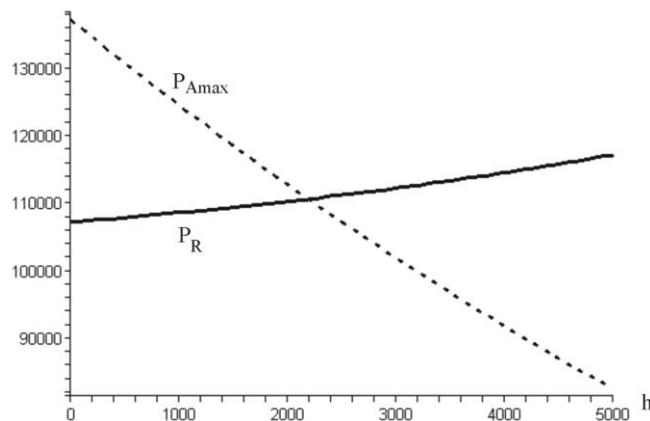
Fig. 2 Required power  $P_R$  and maximum available power  $P_{Amax}$  as a function of altitude  $h$ , for the climbing airplane CP-1 at 20°, with a constant speed of 25 m/s
