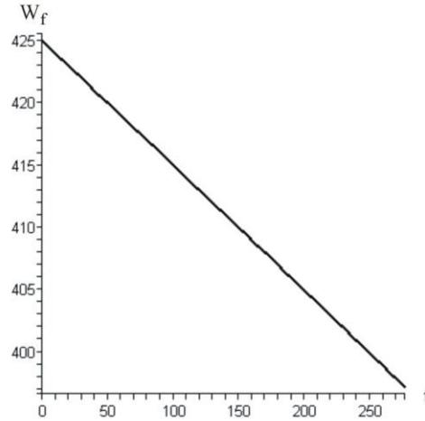
Fig. 6 Fuel of the CP-1 airplane as it climbs at  $20^\circ$ , with the initial speed of 25 m/s, up to 2335 m, with a constant Mach number of 0.0735.
