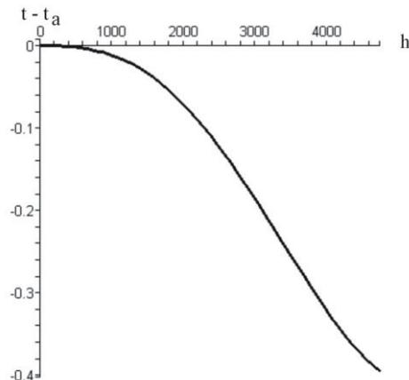
Fig. 8 The error  $t(h) - t_a(h)$  as a function of the altitude  $h$ , for a climb of the CP-1 airplane at  $10^\circ$ , climbing from sea level with a speed of 25 m/s, up to 4748 m
