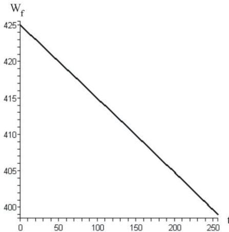
Fig. 1 Fuel of the CP-1 airplane as it climbs at 20°, at the speed of 25 m/s, up to 2190 m
