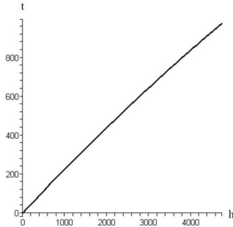
Fig. 7 Time as a function of altitude, for the CP-1 airplane climbing at  $10^\circ$ , starting at the speed of 25 m/s, up to 4748 m
