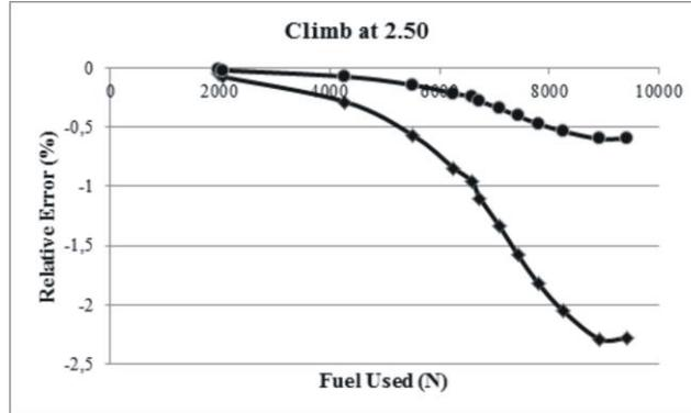
Fig. 4 Relative error in the approximation of the amount of fuel in % for a 2.5° climb-angle of the Hercules-Like airplane, in terms of the total fuel used in the trajectory. The curve with the square markers and that with the round markers correspond respectively to the one-step and the two-step linear approximation.
