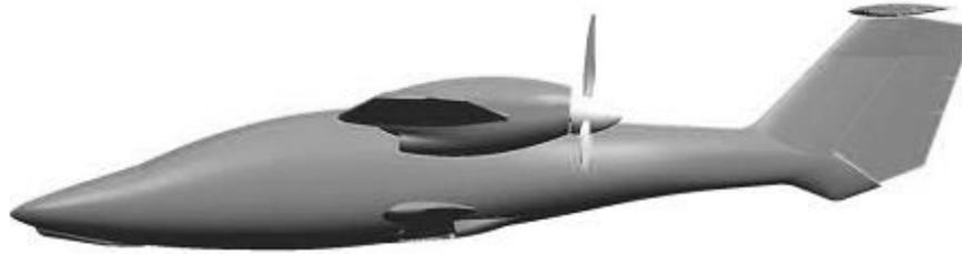
Fig. 1 BE1 pusher aircraft configuration
