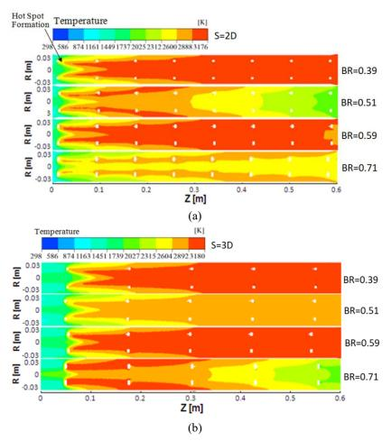
Fig. 7 Contours of detonation wave propagation temperature in detonation tube with obstacle for spacing of (a) S=2D and (b) S=3D
