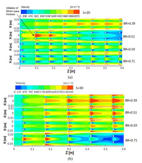
Fig. 6 Contours of detonation wave propagation velocity in detonation tube with obstacles for spacing (a) S=2D and (b) S=3D
