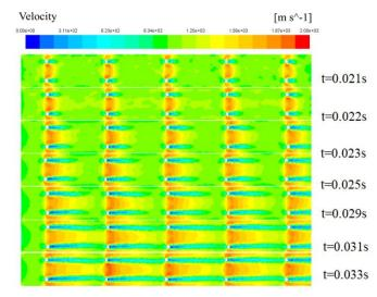
Fig. 4 Detonation wave propagation velocity in detonation tube for several pulse times
