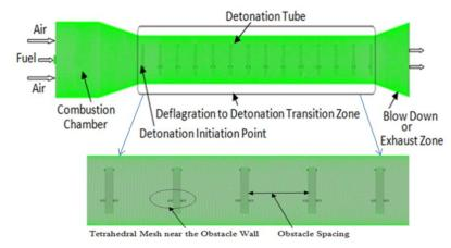
Fig. 2 Tetrahedral mesh of combustion domain with obstacles
