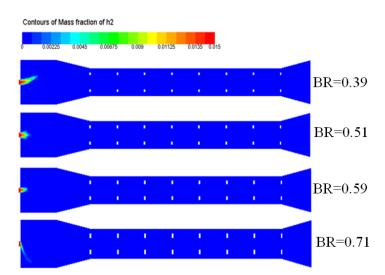
Fig. 5 Hydrogen species mass fraction contour of combustion product in detonation tube with obstacles effect
