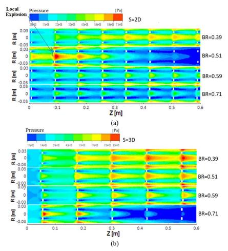
Fig. 8 Contours of detonation wave pressure in detonation tube with obstacles for spacing (a) S=2D and (b) S=3D
