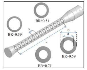
Fig. 1 The physical model of PDE combustor with array of obstacle
