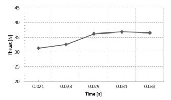
Fig. 12 Propulsive thrust variation in PDC with different pulse time
