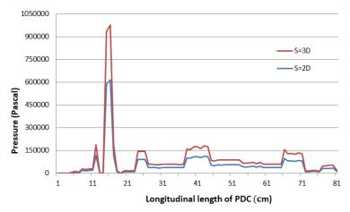
Fig. 11 Detonation wave pressure fluctuation at different wave traveling distance in detonation tube at pulse time of 0.031s
