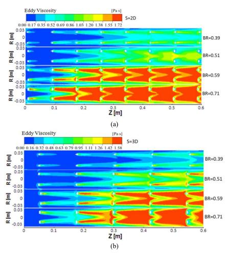
Fig. 9 Contours of eddy viscosity of reacting mixture in obstacle landed detonation tube with blockage for spacing (a) S=2D and (b) S=3D
