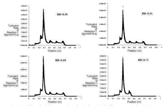
Fig. 10 Variation of turbulence rate of reaction in channel with different obstacles for S=12 cm
