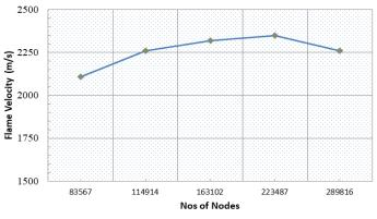
Fig. 3 Grid independence test of computational domain
