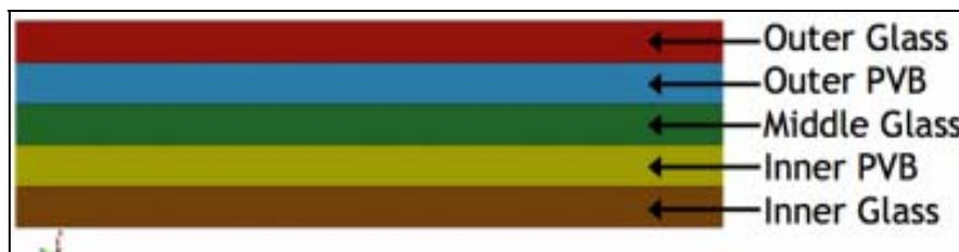
Fig. 3 Windshield lay-up configuration
