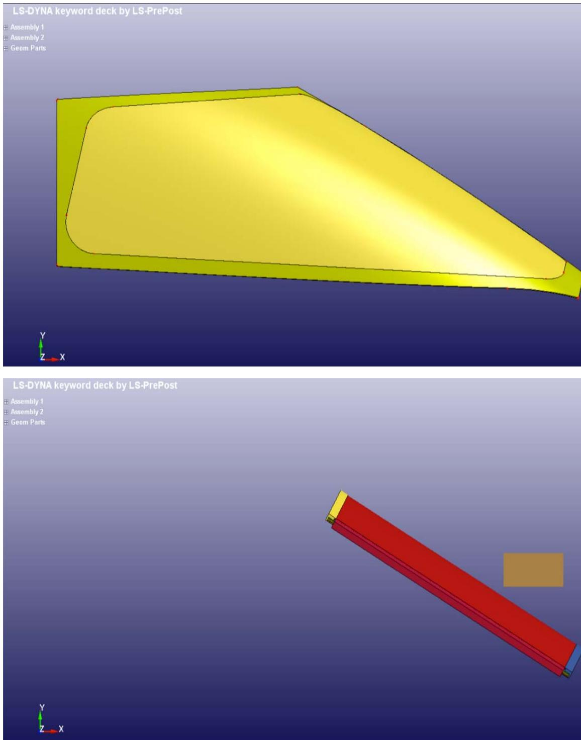
Fig. 9 Full-scale and simplified windshield models
