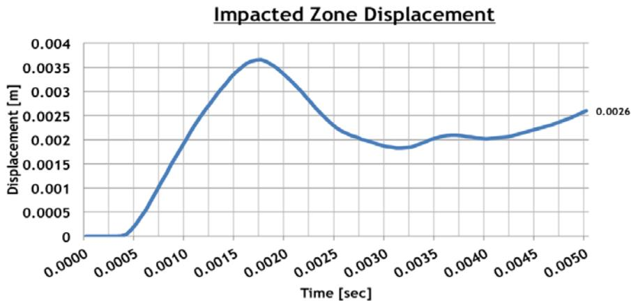
Fig. 13 Displacement of the impacted zone of the right panel
