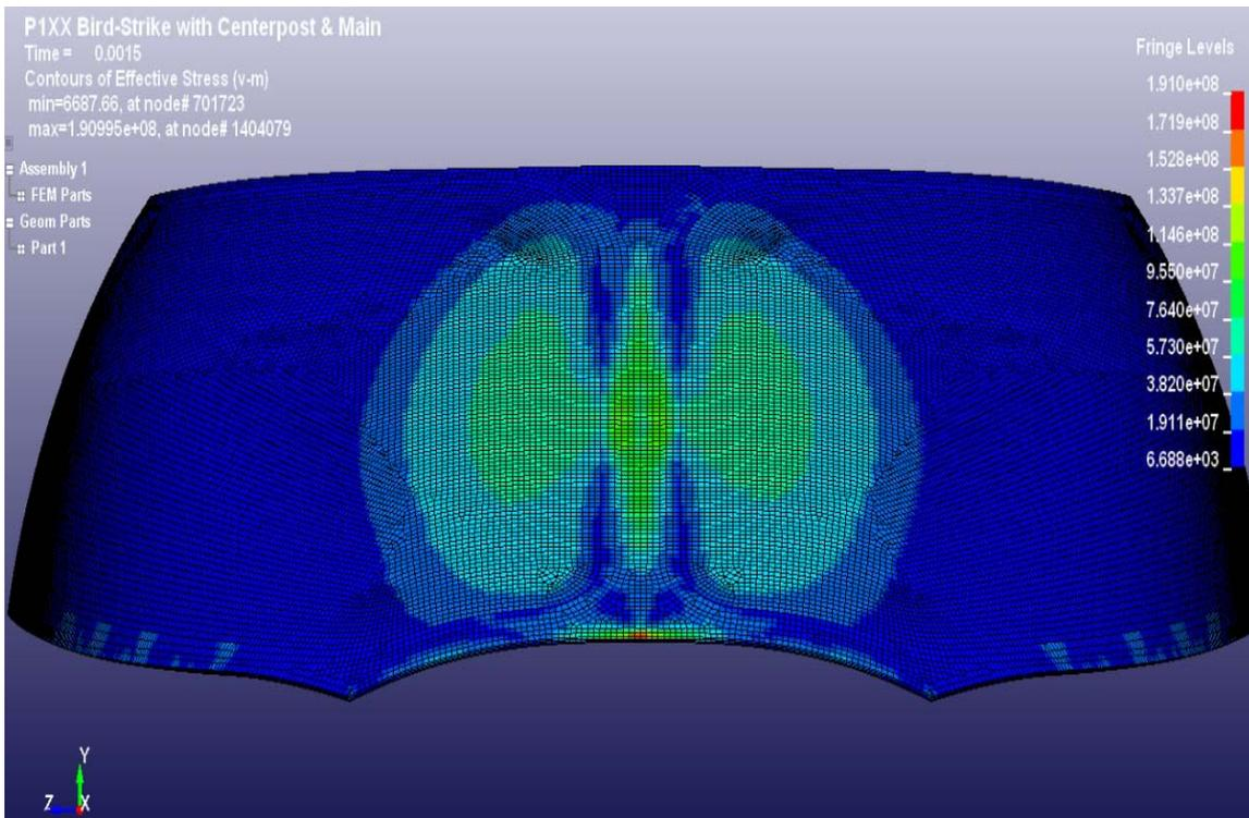
Fig. 17 Von Mises stress plot for birdstrike vs the center beam
