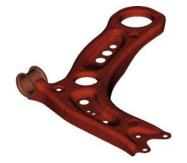
Fig. 13 FE model of the track control arm
