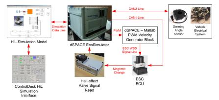
Fig. 7 Tofaş hardware-in-the-loop vehicle simulator for ESC testing
