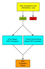
Fig. 16 The flow chart for ESC acceptance and evaluation criterion
