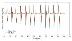
Fig. 13 Change of vehicle yaw rate over time for FMVSS No. 126
