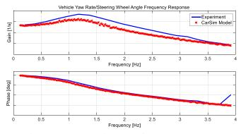
Fig. 5 Yaw rate/steering angle frequency response
