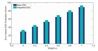
Fig. 21 Error based ESC evaluation scores for FMVSS No. 126 test using different weights
