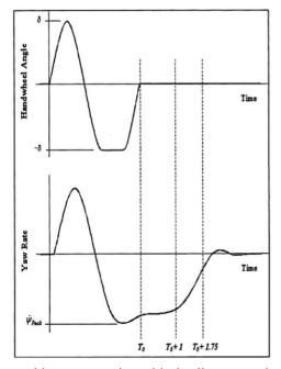
Fig. 9 Vehicle yaw rate change with respect to sine-with-dwell type steering angle input (NHTSA 2007)
