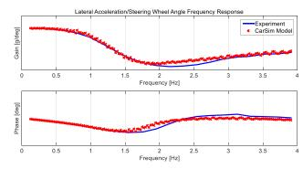
Fig. 4 Lateral acceleration/steering angle frequency response
