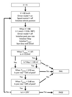
Fig. 10 The flow chart of FMVSS No. 126 test (CarSim 2011)
