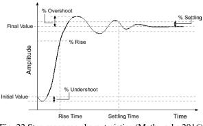
Fig. 22 Step response characteristics (Mathworks 2016)
