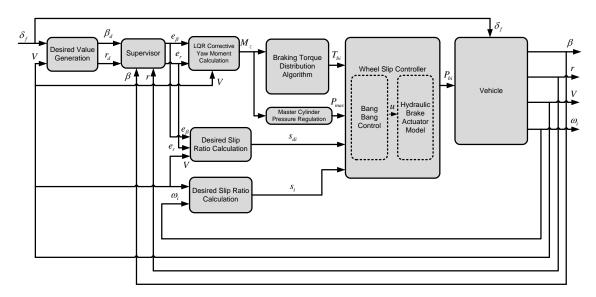
Fig. 18 The Integrated ESC system block diagram
