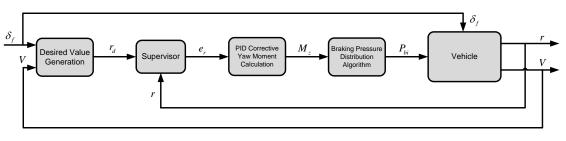
Fig. 17 The Basic ESC system block diagram
