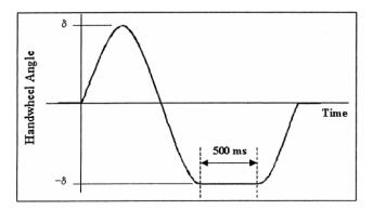
Fig. 8 Sine-with-dwell steering input used in FMVSS No.126 test (NHTSA 2007)
