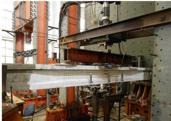
Fig. 3 Test setup for monotonic and fatigue loading
