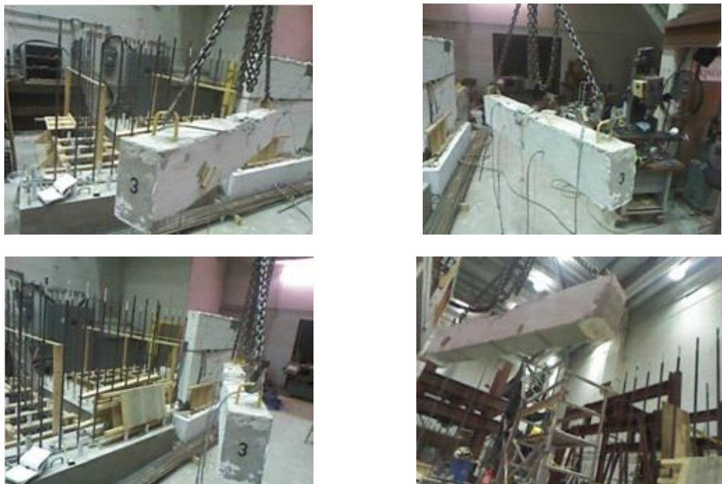
Fig. 2 (a) – (d) 2D images of Reinforced Concrete beams (for 3D model development)
