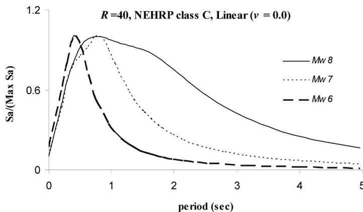
Fig. 5 Effect of the earthquake's magnitude on the response spectra when the COV of the moment magnitude, distance, and other variables are assumed to equal 0.02, 0.10, and 0.20, respectively. The response spectra were normalized by the peak response spectra to compare the spectral shape
