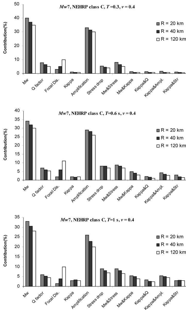
Fig. 7 The relative contributions to the response for distances of 20, 40 and 120 km at periods of 0.3, 0.6, and 1.0 s when the COV of the moment magnitude, distance, and other variables are assumed to equal 0.02, 0.10, and 0.15, respectively
