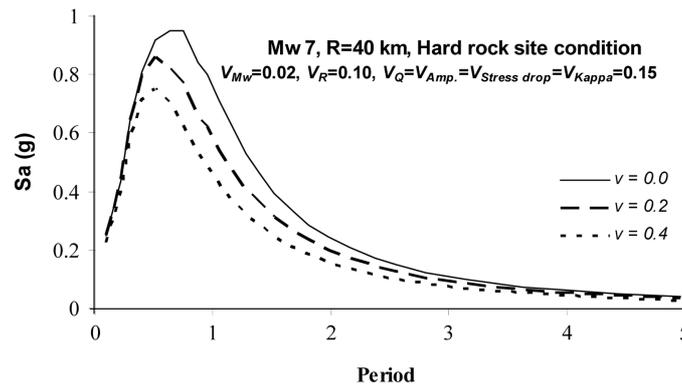
Fig. 2 The probabilistic mean values of the response spectra for different coefficients of structural nonlinearity
