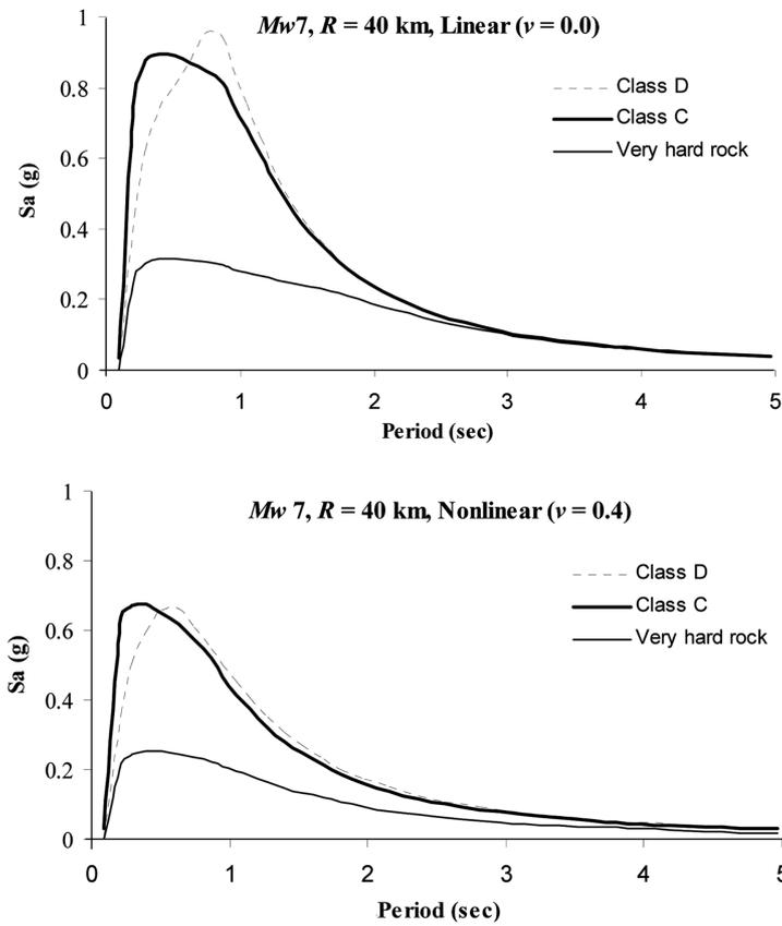
Fig. 4 Comparison of the linear and nonlinear response spectra for different site conditions when the COV for the moment magnitude, distance, and other variables are assumed to equal 0.02, 0.10, and 0.15, respectively
