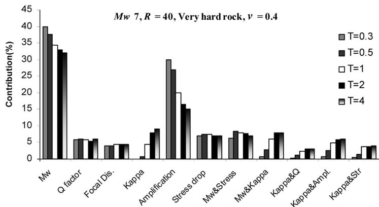
Fig. 10 The relative contributions to the response in the SDOF system at different periods when the COV of the moment magnitude, distance, and other variables are assumed to equal 0.02, 0.10, and 0.15, respectively
