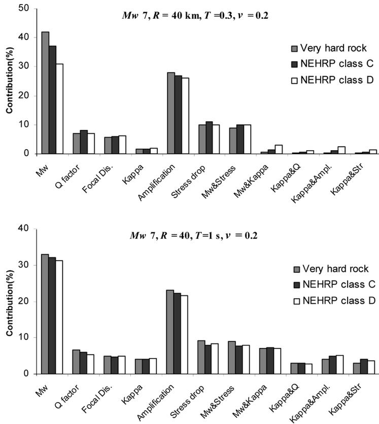
Fig. 9 The relative contributions at periods of 0.3 and 1.0 s for three groups of soil conditions when the COV of the moment magnitude, distance, and other variables are assumed to be equal to 0.02, 0.10, and 0.15, respectively
