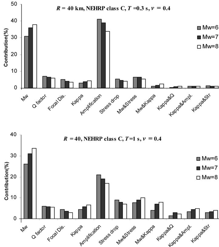
Fig. 8 The relative contribution that was computed for three different magnitudes when the COV of the moment magnitude, distance, and other variables are assumed to equal 0.02, 0.10, and 0.15, respectively
