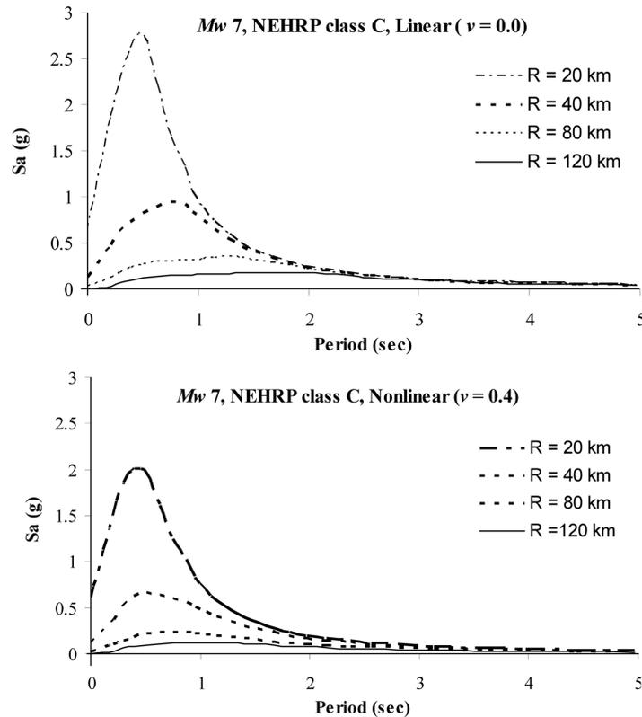
Fig. 3 Comparison of the linear and nonlinear acceleration response spectra in four different distances when the COV of the moment magnitude, distance, and other variables are assumed to equal 0.02, 0.10, and 0.12, respectively
