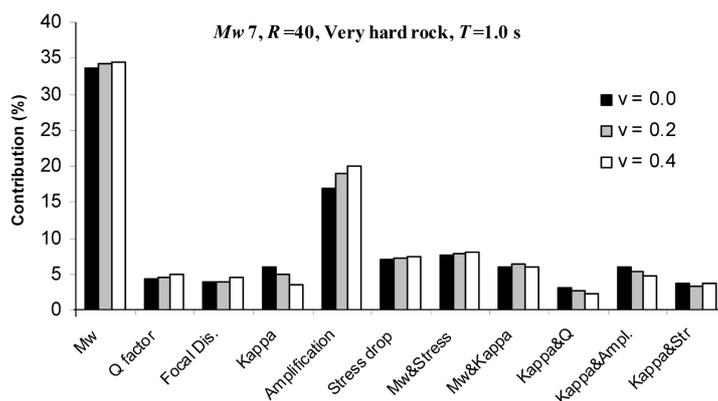
Fig. 6 Relative contributions of the variances in variables and the covariance between them to the variance in the response in the SDOF system when the distance takes the value of 40 km and  $M_w$  7 at a period of 1 s for different nonlinearity when the COV of the moment magnitude, distance, and other variables are assumed to equal 0.02, 0.10, and 0.15, respectively
