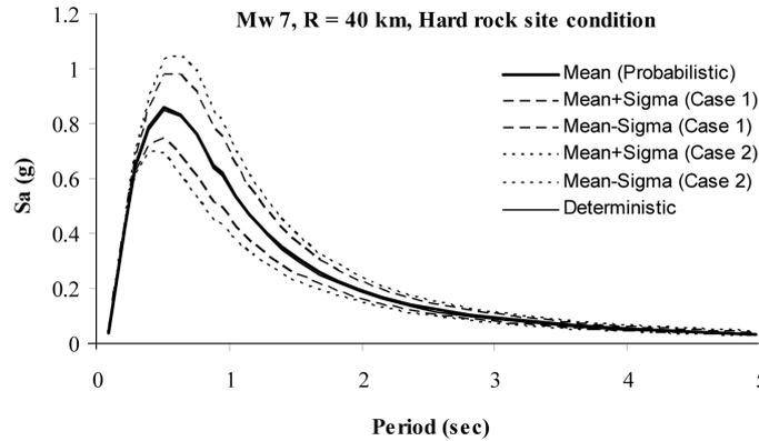
Fig. 1 Comparison of the mean value obtained with the probabilistic and deterministic methods. The dashed lines show the effect of the standard deviation for the following cases: Case 1)  $V_{Mw} = .02$ ,  $V_R = 0.10$ ,  $V_Q = V_{Amp} = V_{Kappa} = V_{Stress\ drop} = 0.12$  and Case 2)  $V_{Mw} = 0.02$ ,  $V_R = 0.10$ ,  $V_Q = V_{Amp} = V_{Kappa} = V_{Stress\ drop} = 0.20$
