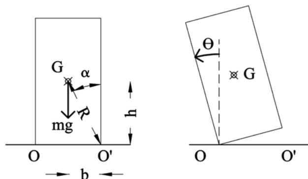
Fig. 1 Parameters describing Housner model of a rigid body and its displacement.
