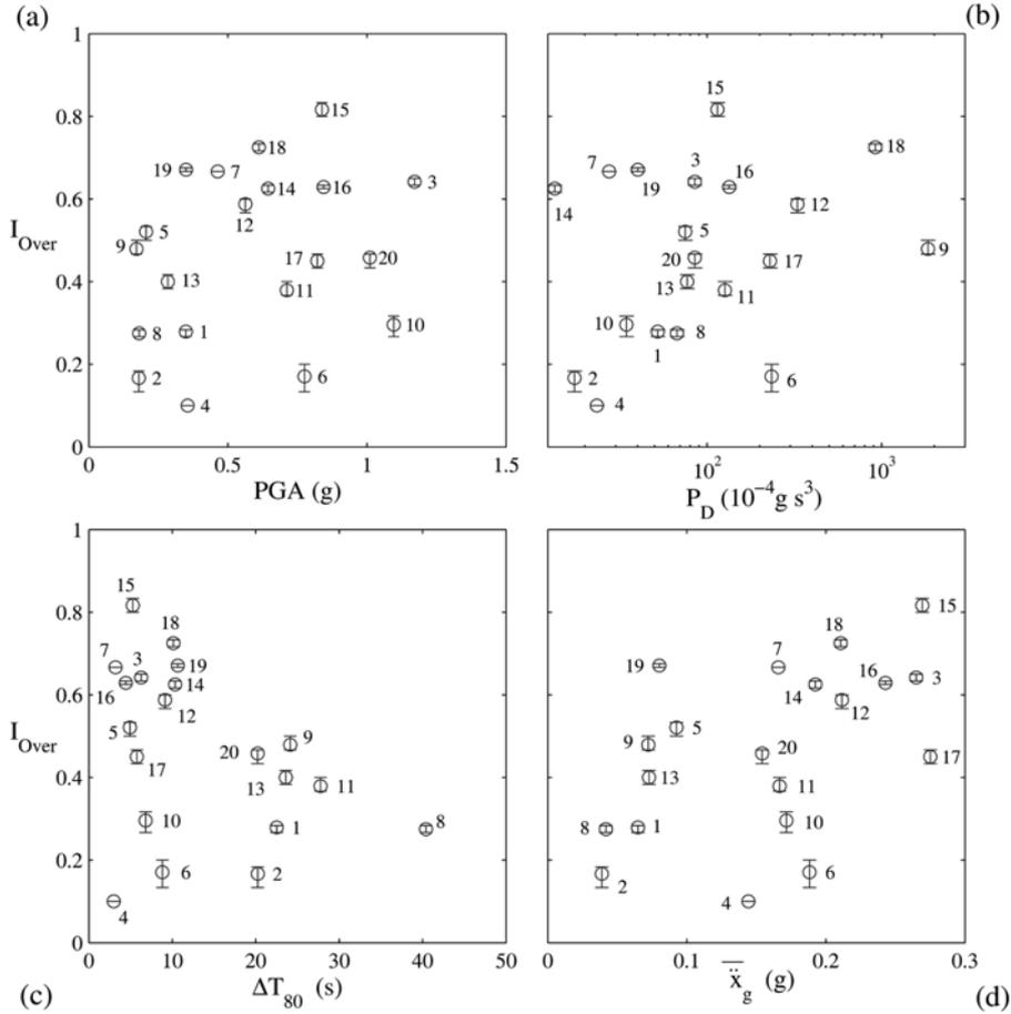
Fig. 8 For  $\bar{R} = 3$  m and unscaled PGA, correlation between the mean value and the interquartile range of the Overturning Index of Eq. (4) and PGA (a), destructiveness potential of Eq. (5) (b), Significant Duration (c), root mean square acceleration (d). Numbering refers to signals as reported in Table 1.
