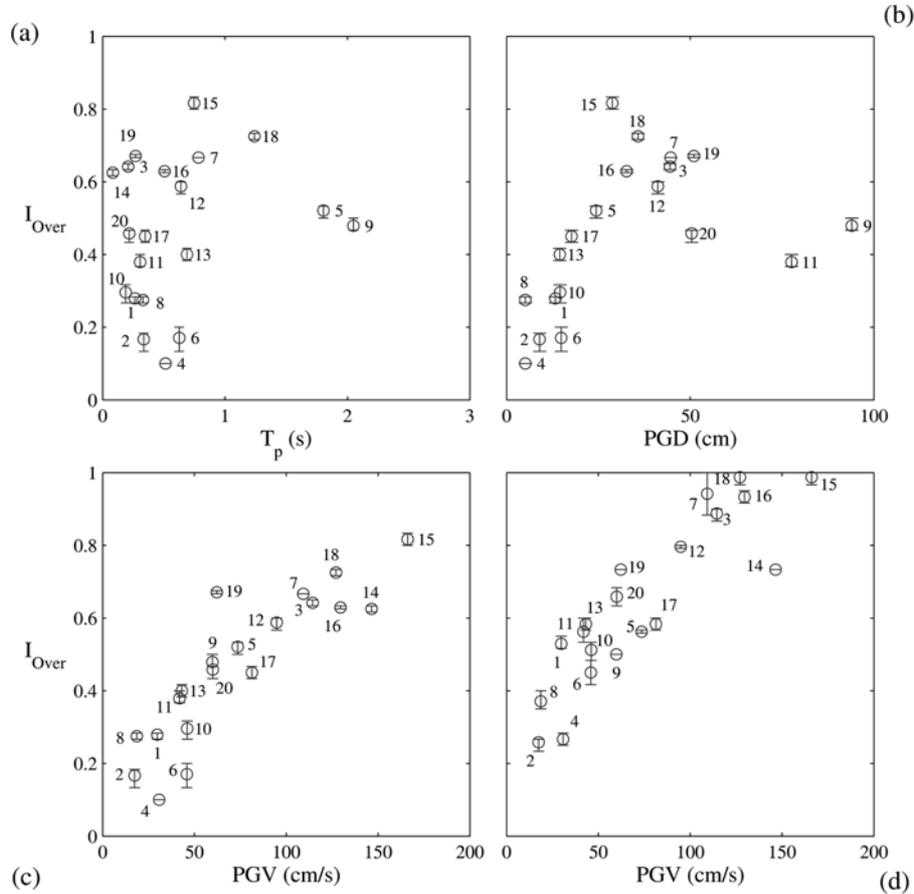
Fig. 9 For unscaled PGA, correlation between the mean value and the interquartile range of the Overturning Index of Eq. (4) and predominant period ( $\bar{R} = 3$  m) (a), PGD ( $\bar{R} = 3$  m) (b), PGV ( $\bar{R} = 3$  m) (c) and PGV ( $\bar{R} = 1.5$  m) (d). In figure (b) the PGD of the record LucN80W is not represented, because out of range. Numbering refers to signals as reported in Table 1.
