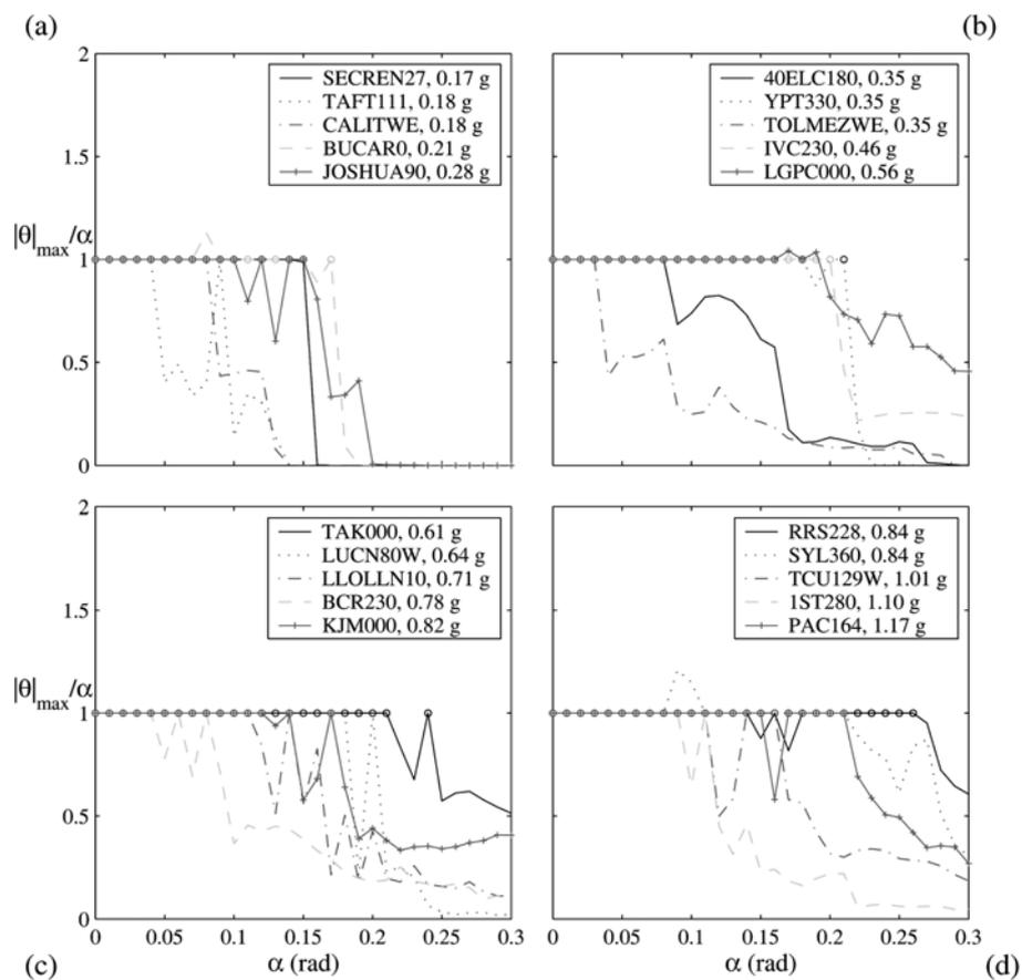
Fig. 7 For  $R = 3$  m, rocking curves in terms of normalised maximum absolute rotation to different signals (refer to Table 1), sorted by PGA in ascending order from (a) to (d), as reported in each legend. The circle indicates an overturning.
