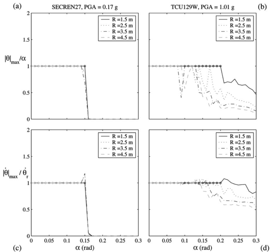
Fig. 4 Rocking curves as a function of  $\alpha$  and  $R$  in terms of kinematic parameters: (a) and (b) normalised maximum absolute rotation, (c) and (d) normalised maximum absolute angular velocity, for different accelerograms: (a) and (c) SecreN27, (b) and (d) TCU129W, both unscaled (refer to Table 1). The circle indicates an overturning.
