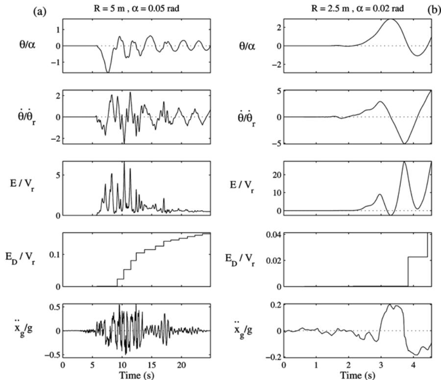
Fig. 3 Sample time histories of, from top to bottom, normalised angular displacement and velocity, mechanical energy, dissipated energy and ground acceleration. Accelerograms: (a) LGPC000, (b) BUCAR0 (refer to Table 1).
