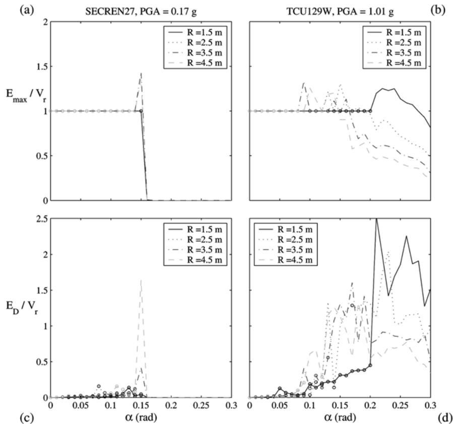
Fig. 5 Rocking curves as a function of  $\alpha$  and  $R$  in terms of energy parameters: (a) and (b) normalised maximum mechanical energy, (c) and (d) normalised dissipated energy, for different accelerograms: (a) and (c) SecreN27, (b) and (d) TCU129W, both unscaled (refer to Table 1). The circle indicates an overturning.
