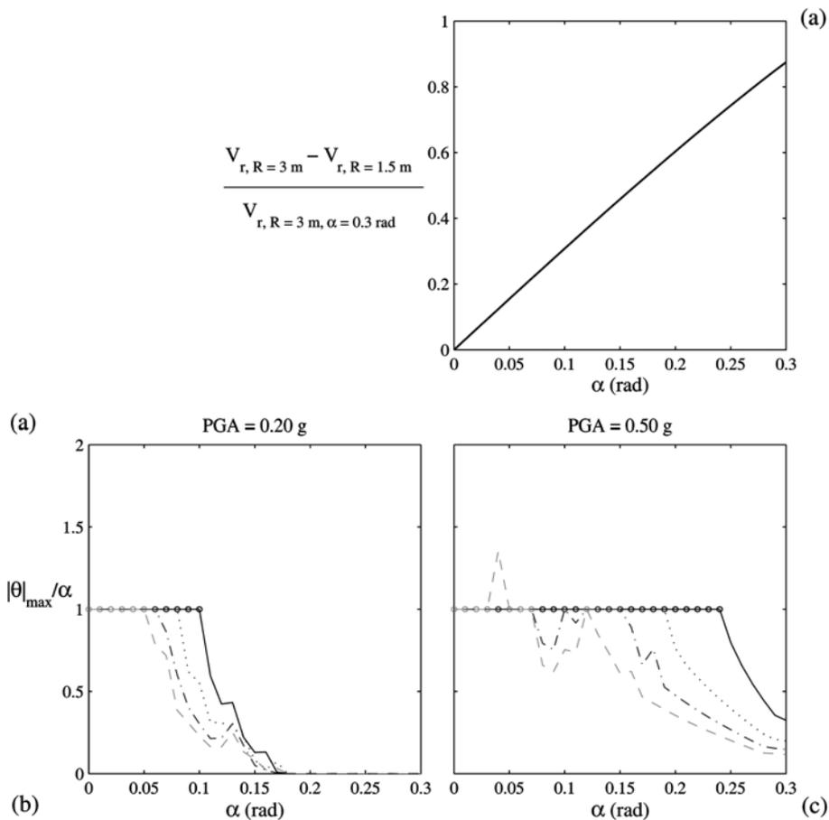
Fig. 6 Tangibility of the scale effect. (a): normalised difference of reference potential energy  $V_r$  of two blocks with same angle  $\alpha$ , but different length  $R$ . (b) and (c): rocking curves as a function of  $\alpha$  and  $R$  in terms of normalised maximum absolute rotation for the same accelerogram, RRS228 (refer to Table 1), scaled to different PGA: 0.2 g (b) and 0.5 g (c). The circle indicates an overturning.
