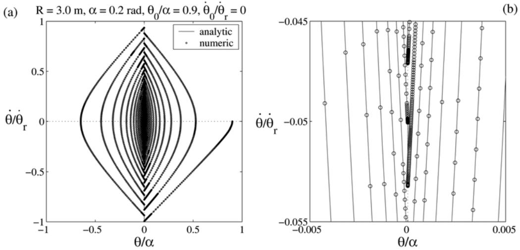
Fig. 2 Comparison of analytic (closed form) solution and numeric integration for free vibration. (b) is a zoom of (a).
