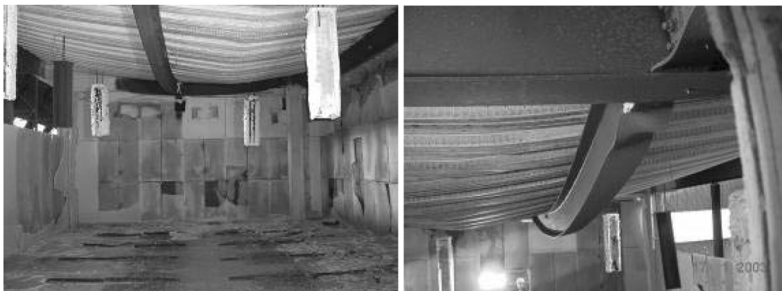
Fig. 6 7 th Cardington fire test - compartment after fire, residual deformation 925 mm, no local collapse of structure
