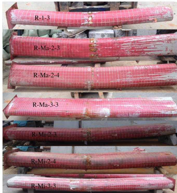
Fig. 4 Typical failure modes for all tested specimens
