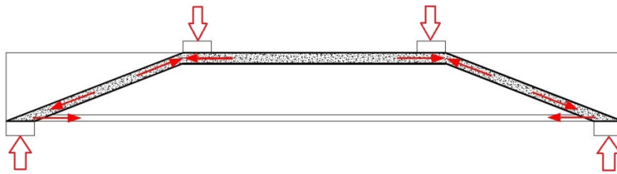
Fig. 25 Tied-arch model on the core concrete
